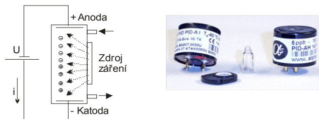
Fig. 6 Principle and real pieces of photo-ionization sensors of VOC
