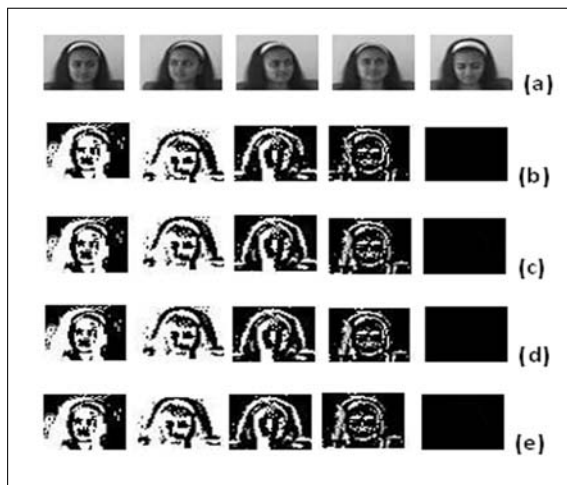
Fig. 10. (a) Female images and eigen faces using (b) Double precision floating-point (c) 24-bit, (d) 32-bit and (e) 64-bit fixed-point
