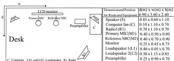
Fig. 19 Test environment (left) and room dimension, locations of sound source and equipment (right)
