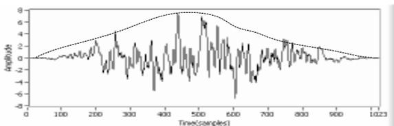
Fig. 4 Example of short segmented (windowed) signal
