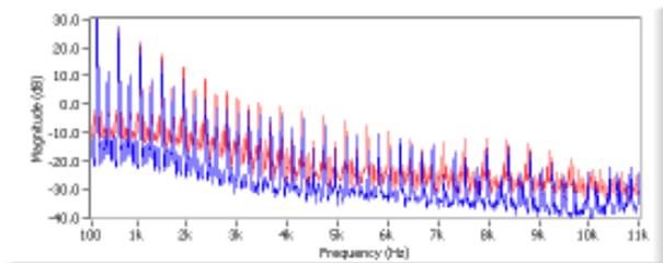
Fig. 22 Comparison of omnidirectional (top waveform) and unidirectional (bottom) microphone on echo sound
