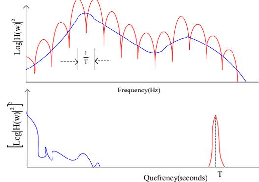
Fig. 1 Example of logarithmic power spectrum (top) and its power spectrum (bottom)
