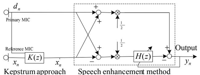
Fig. 18 Block diagram of G-J kepstrum adaptive beamformer
