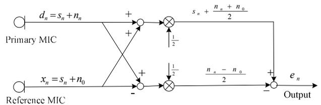
Fig. 16 Block diagram of typical beamforming method
