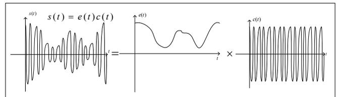
Fig. 2 The signal  $s(t)$ , envelope  $e(t)$  and carrier  $c(t)$
