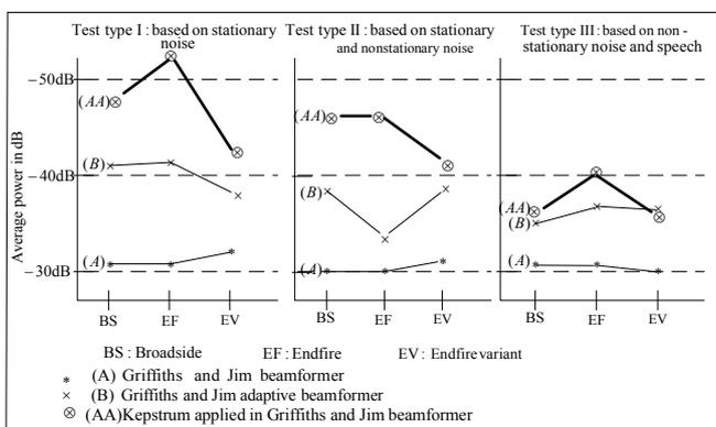
Fig. 26 Comparison of performance based on different microphones set-up
