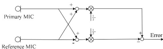
Fig. 13 Block diagram of G-J beamformer
