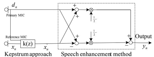
Fig. 17 Block diagram of G-J kepstrum beamformer
