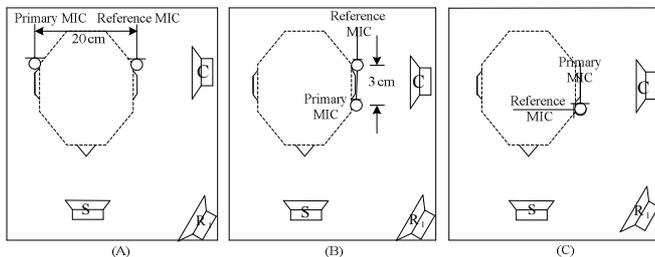
Fig. 25 Experimental microphone set-up (S: speaker, C: computer fan noise, R: radio noise):
