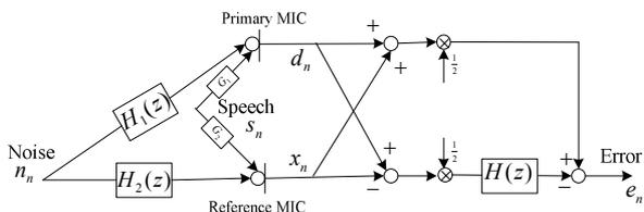
Fig. 15 Block diagram of basic speech enhancement method
