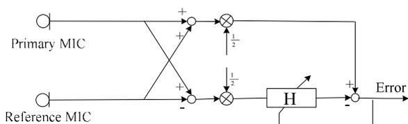
Fig. 14 Block diagram of G-J adaptive beamformer
