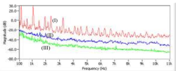
Fig. 23 (I) G-J beamformer (II) G-J adaptive beamformer (III) G-J kepstrum beamformer
