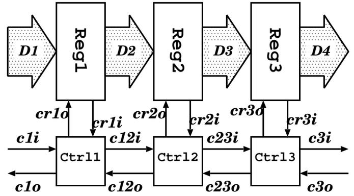
Fig. 9. An asynchronous pipeline.
