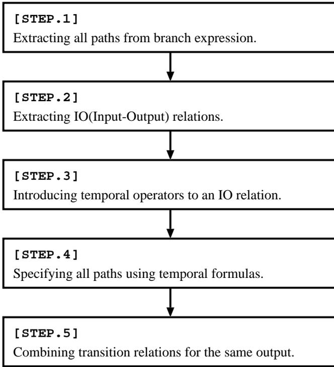
Fig. 6. Procedure of Specification.
