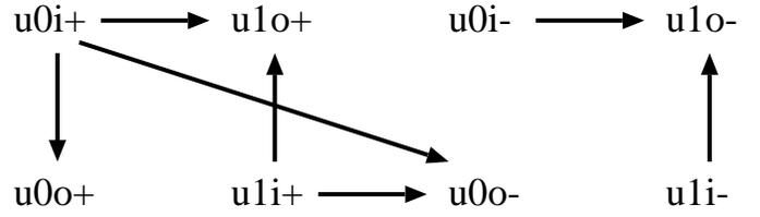
Fig. 7. A reduced signal transition graph for Fig.3 by check-points extraction method
