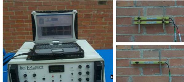
Fig. 3. The MsS 2020@ system and its transducer sensor
