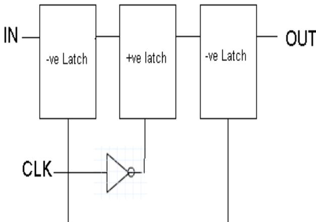
Fig.9 One bit shift register block.
