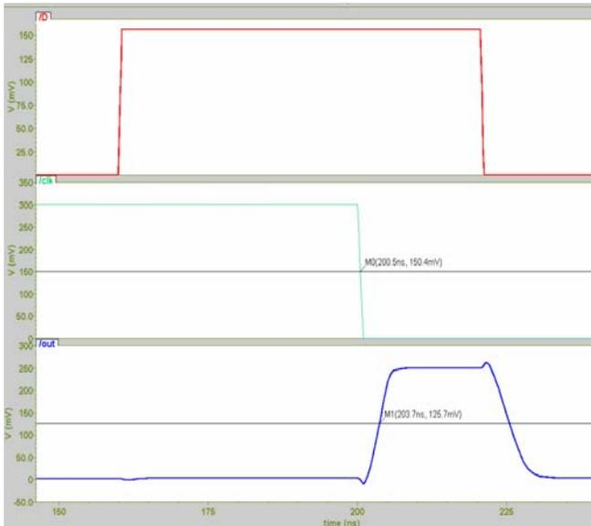
Fig.8 negative latch delay
