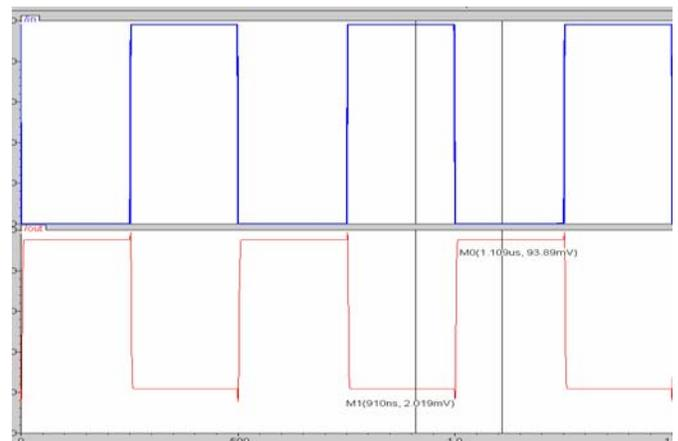
Fig.3 the output waveform of the low threshold inverter in the sub-threshold region.
