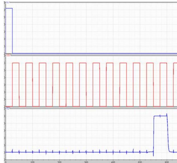
Fig.13 waveform of 10-bit Shift Register at 30 KHz clock frequency and 30% activity
