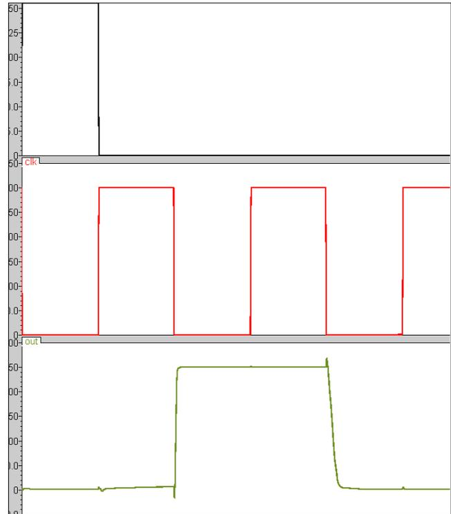
Fig.10 waveform of one bit shift register
