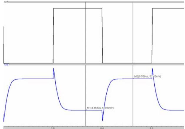
Fig.5 waveform of high-threshold inverter in the sub-threshold region.
