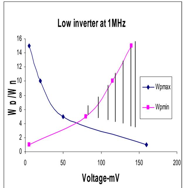
Fig.2 Sizing low threshold inverter for min  $V_{dd}$
