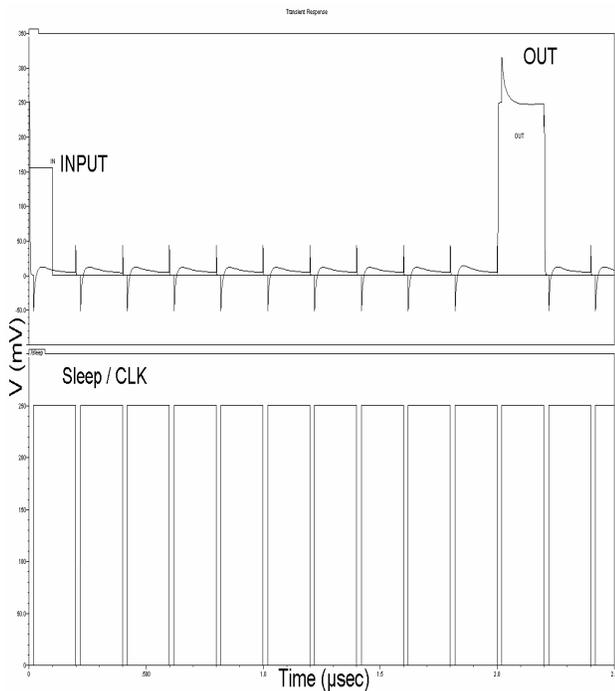
Fig.12 waveform of 10-bit Shift Register at 5 MHz clock frequency and 10% activity
