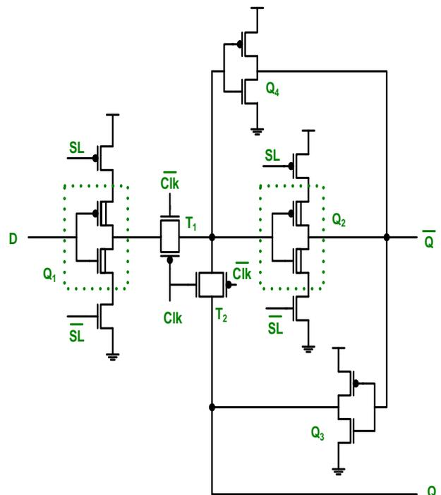
Fig.6 Schematic of the MTCMOS low power Latch
