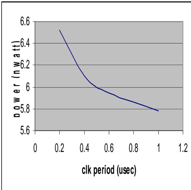
Fig.1 Trade off between the power consumption and the propagation delay.
