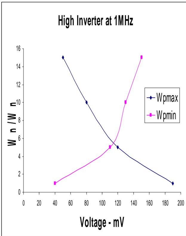
Fig.4 Sizing high threshold inverter for min  $V_{dd}$
