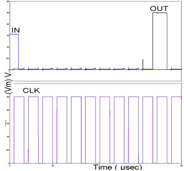
Fig.11 waveform of 10-bit Shift Register at 30 KHz clock frequency and 30% activity
