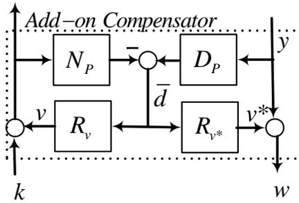
Fig. 6 Structure of the add-on compensator
