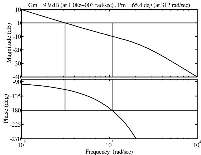
Fig. 11 Frequency response characteristics of the systems
