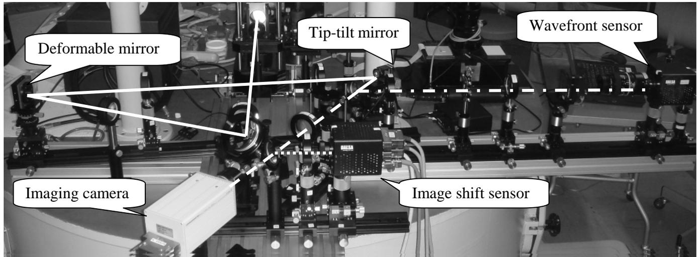
Fig. 12 Photograph of the optical setup of the AO system
