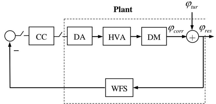
Fig. 2 Block diagram of the AO system
