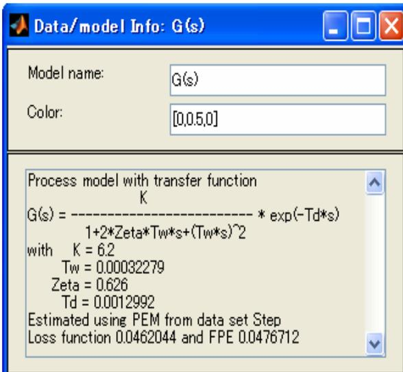
Fig. 3 System Identification result of the plant modeling structure
