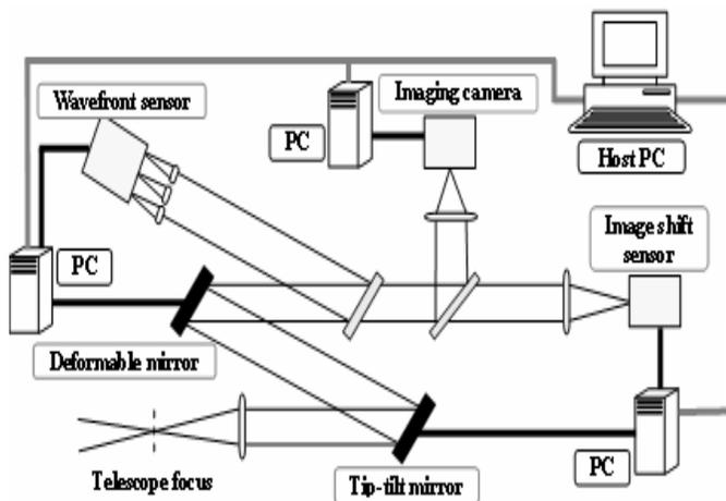
Fig. 1 Hardware structure of the AO system
