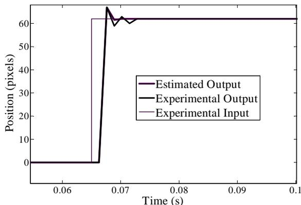
Fig. 4 Step input responses of real and estimated plant
