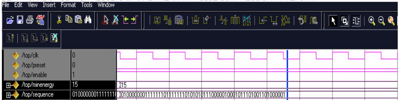
Fig. 3 Behavioral simulation result of a good 31-bit Ternary Pulse compression sequence.
