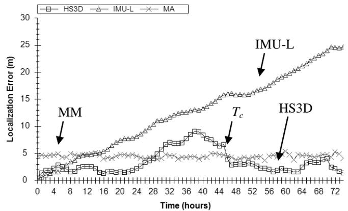
Fig. 7. Localization Error of HS3D, IMU-L and MM algorithms
