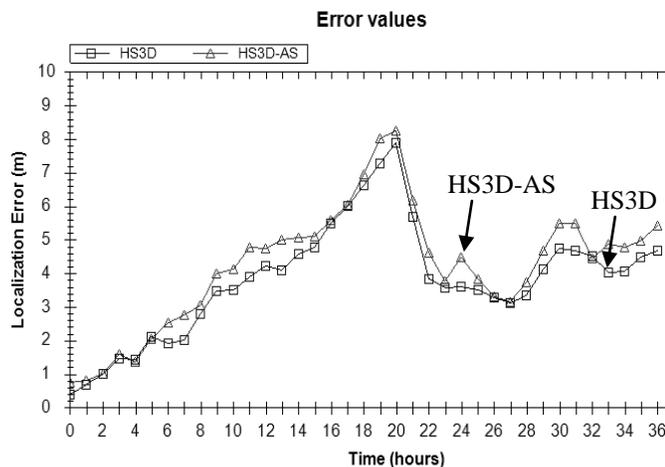
Fig.11 Localization error of HS3D and HS3D-AS algorithms
