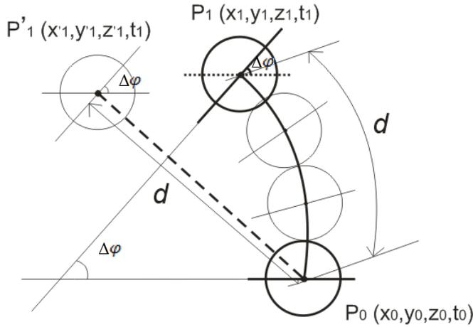
Fig. 5. Trajectory estimation when both rotation and translation.
