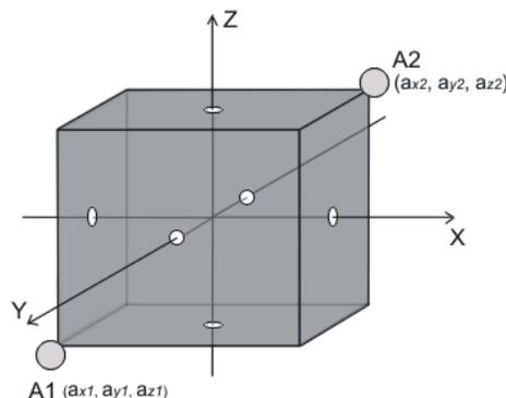
Fig. 1. Cube model for accelerometers' placement
