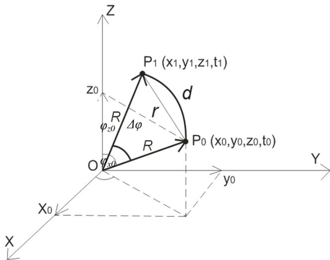
Fig. 6. Translation and rotation of node in 3-D representation
