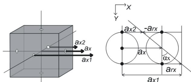
Fig. 2. Translation and rotation acceleration on X-axis
