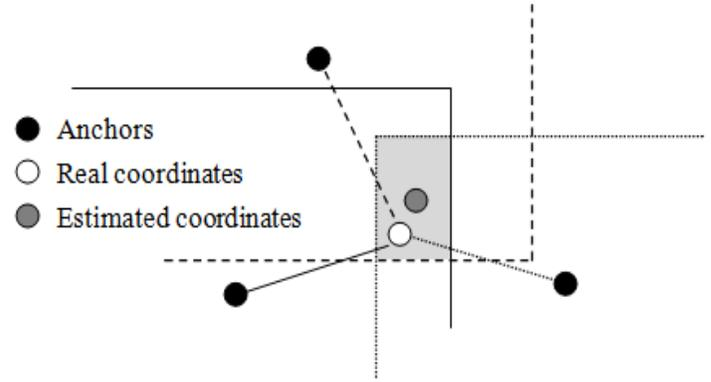
Fig. 3 Min-Max localization algorithm
