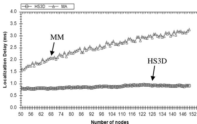
Fig. 8. Localization delay of HS3D and MM algorithms
