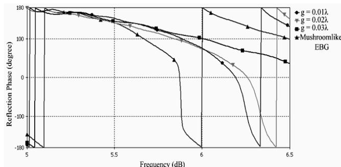
Fig. 4 the results of reflection phases of the EBG structure
