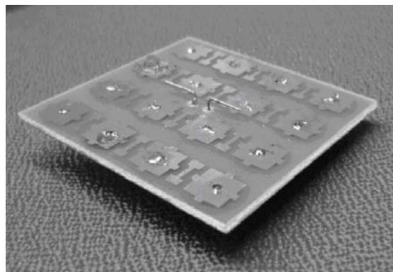
Fig. 22 the prototype of proposed antenna
