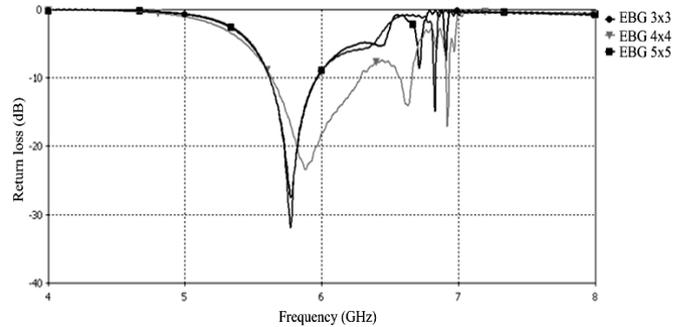
Fig. 5 the return loss of wire dipole above novel EBG reflector versus variation of a number of elements
