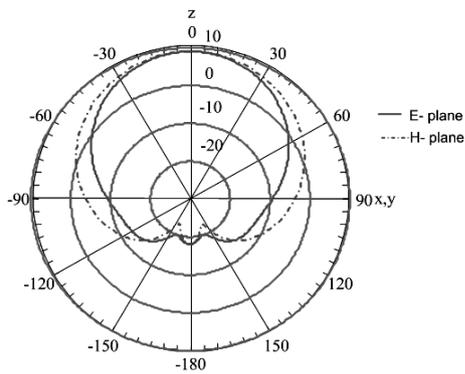
Fig. 11 directive gain of the dipole above novel EBG with distance of  $h_1$  is  $0.02\lambda_{5.8 \text{ GHz}}$
