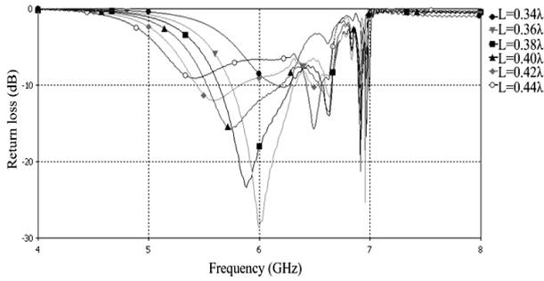
Fig. 10 return loss of the dipole above novel EBG with distance of  $h_1$  is  $0.02\lambda_{5.8 \text{ GHz}}$
