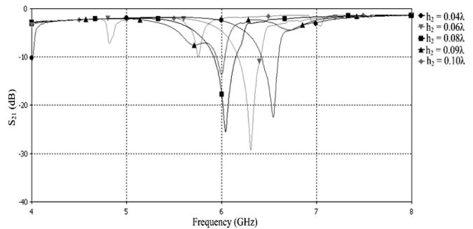
Fig. 18 insertion Loss of the Adjustment of  $h_2$
