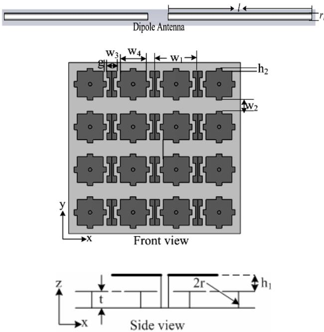
Fig. 1 configuration of wire dipole with novel EBG reflector
