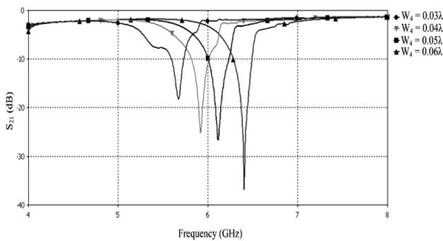
Fig. 17 insertion loss of patch width ( $W_3$ ) with difference sizes.
