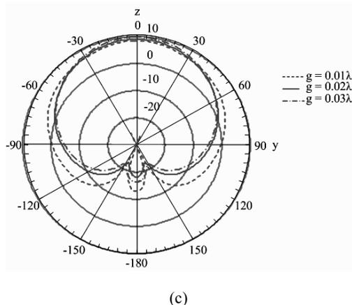
Fig. 19 return loss and radiation pattern of wire dipole above novel EBG reflector with different gap spacing: (a) return loss, (b) E-plane, and (c) H-plane
