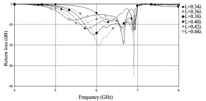
Fig. 13 return loss of the dipole above novel EBG with distance of  $h_1$  is  $0.03\lambda_{5.8 \text{ GHz}}$
