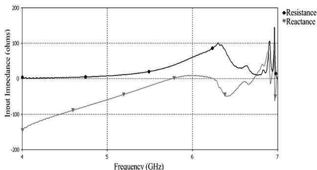
Fig. 20 input impedance of wire dipole above novel EBG reflector
