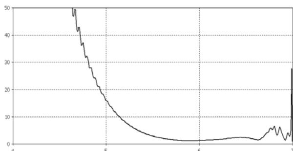
Fig. 21 VSWR of wire dipole above novel EBG reflector
