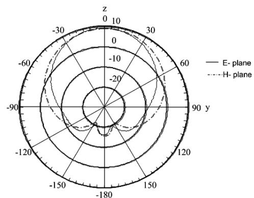
Fig. 14 directive gain of the dipole above novel EBG with distance of  $h_1$  is  $0.02\lambda_{5.8 \text{ GHz}}$
