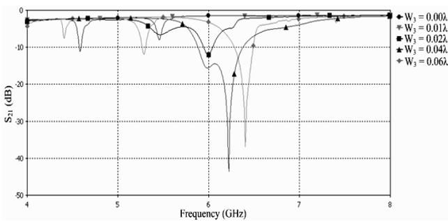
Fig. 16 insertion loss of patch width ( $W_3$ ) with difference sizes
