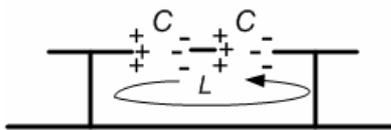
Fig.2 equivalent resonant LC circuit for EBG structure
