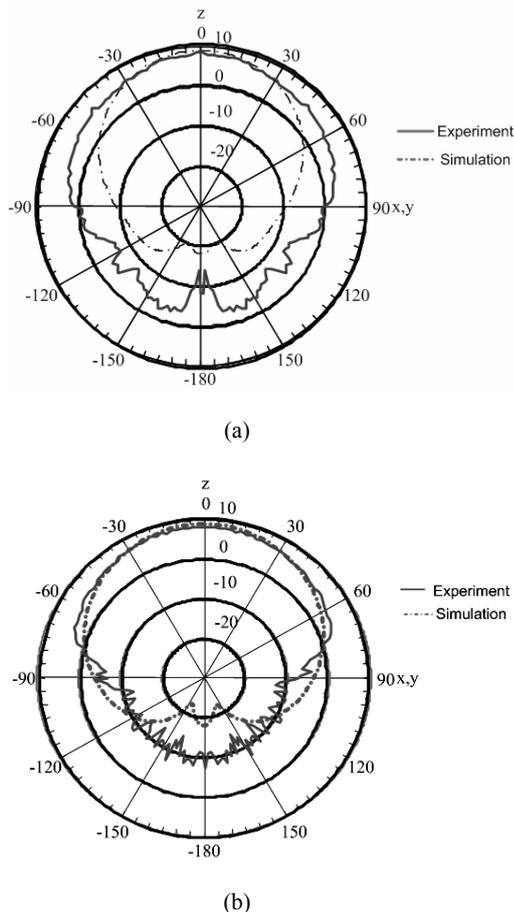
Fig. 24 Radiation pattern of wire dipole above novel EBG reflector: (a) E-plane and (b) H-plane
