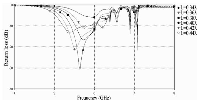
Fig. 7 return loss of the dipole above novel EBG with distance of  $h_1$  is  $0.01 \lambda_{5.8 \text{ GHz}}$
