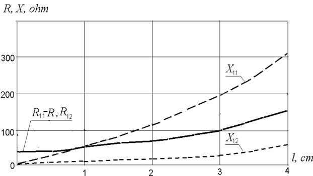
Fig. 8. The self and mutual impedances of the radiators with unequal lengths
