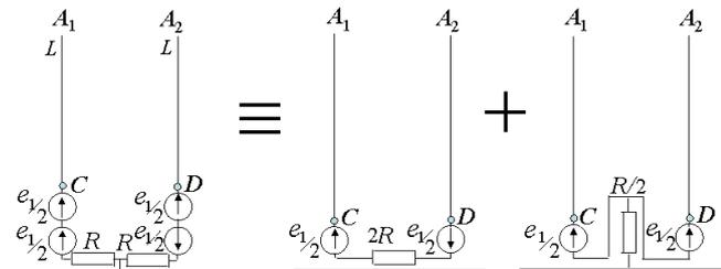
Fig. 3. For calculation of the input impedance
