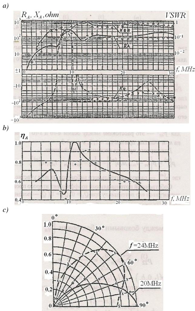
Fig. 10. The input characteristics (a), efficiency (b) and pattern (c) of multi-radiators antenna with complex loading impedance
