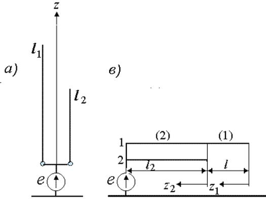
Fig.6. Monopole and equivalent asymmetric line
