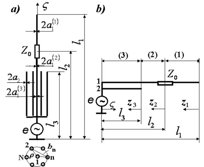
Fig. 9. Multi-radiators antenna with complex loading impedance (a) and an equivalent asymmetrical line (b)
