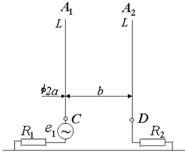
Fig. 2. The two-radiator system
