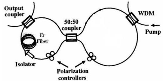
Fig.4: Schematic of a figure of eight fiber laser.
