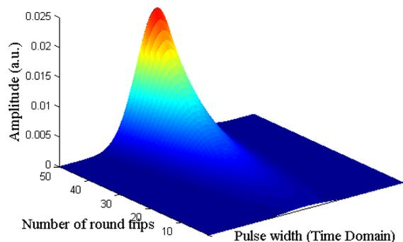
Fig.8: Pulse evolution in figure of eight fiber laser
