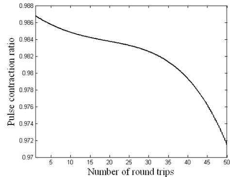
Fig.6: Pulse width ratio at each round trip.
