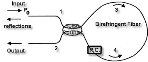
Fig. 3: Schematic of a Nonlinear Optical Loop Mirror.
