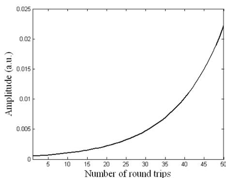
Fig.7: Pulse amplitude at each round trip.
