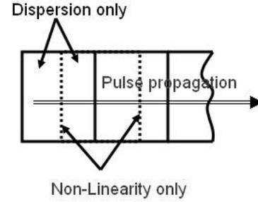
Fig.5: Symmetrized Split Step Fourier Method (SSSFM).
