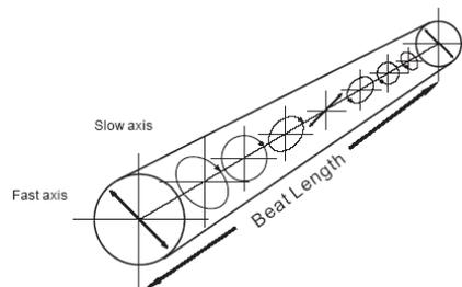
Fig. 1: A schematic diagram of how the polarization varies along a birefringent fibre when the input was polarized at  $45^\circ$  to one axis.
