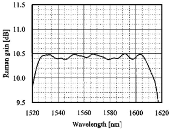
Fig. 2 Measured gain profile (typical) of Raman gain using a multi-pump scheme [12]
