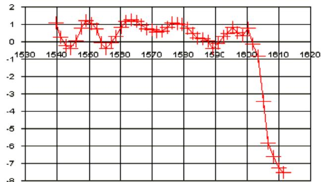
Fig. 6 Typical spectrum of  $NF_{eq}^{dB}$  in forward-pumped case (signal to signal and signal-ASE interactions are not considered)
