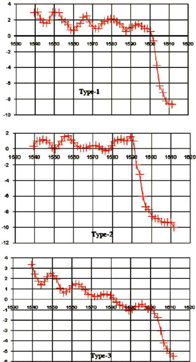
Fig. 7 Spectrum of  $NF_{eq}^{dB}$  for 0dBm input signal power for three types of DRA
