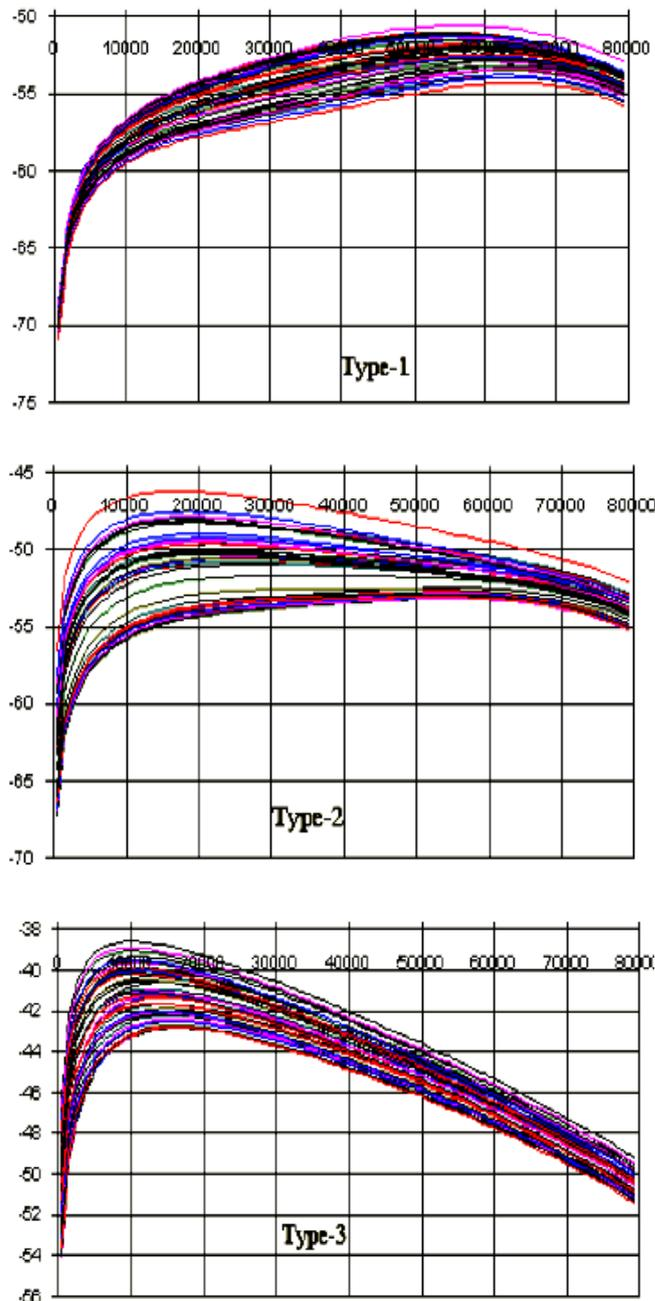
Fig. 4 DRB light power for a typical fibre-pumped DRA
