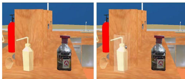
Fig. 2 visual feedback for direct manipulation to drag objects in X, Y and Z axis direction.
