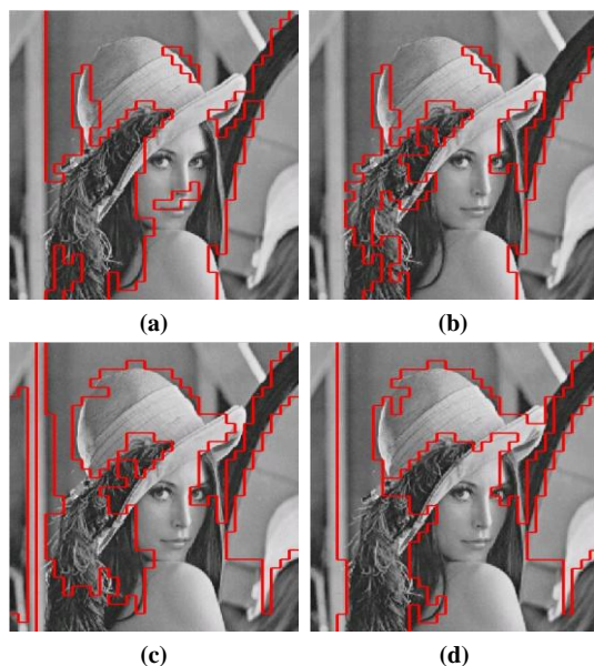
Figure 6 Image segmented into 5 regions with minimal region size of 15 blocks and initial block size of 8x8. The numbers of DCT coefficients for energy calculation are: a) 10 with 1.39s. b) 20 with 1.35s. c) 30 with 1.45s. d) 40 with 1.35s.
