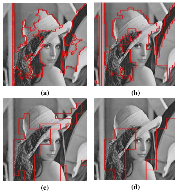
Figure 7 Image segmented into 5 regions with minimal region size of 15 blocks, 50% DCT coefficients are selected while use blocks of size a) 4x4 with 18.83s. b) 8x8 with 1.42s. c) 16x16 with 0.23s. d) 32x32 with 0.064s.
