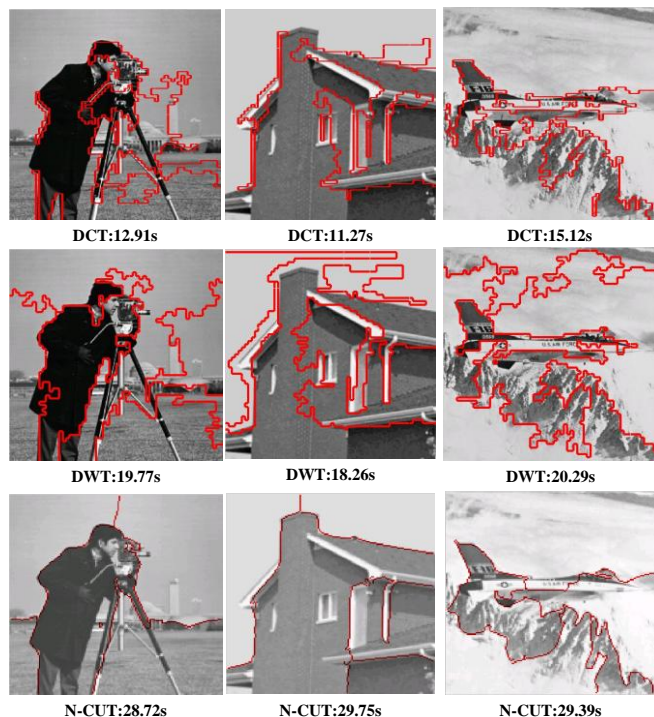
Figure 8 Result of different image segmentation approaches. We adopt the best parameters for our texture segmentation and DWT based approach. First row: our DCT based segment. Second: DWT based segment. Third row: Normalized cut approach. 5 regions are segmented in all the experiments, and the time cost is shown under each example.
