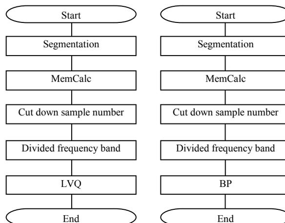
Fig.5: The differences between the proposed method and the method using MEM and BP
