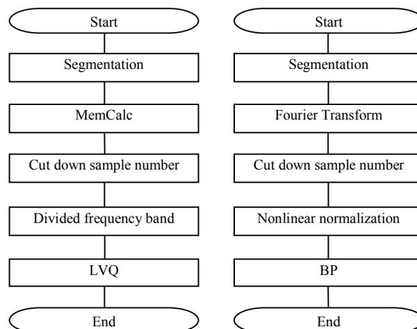
Fig.3: The differences between the proposed method and the method by Inagaki et al.
