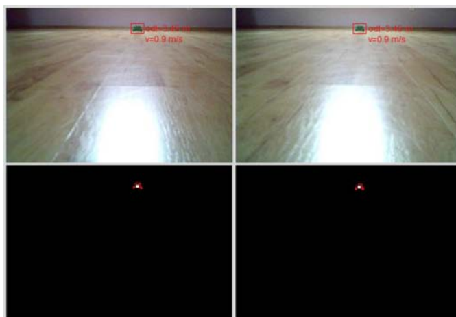
Fig. 9. Calculation of movement parameters of object, detection of moving (object is moving in perpendicular line to the optical axis of cameras with speed of 0.4 m/s)
