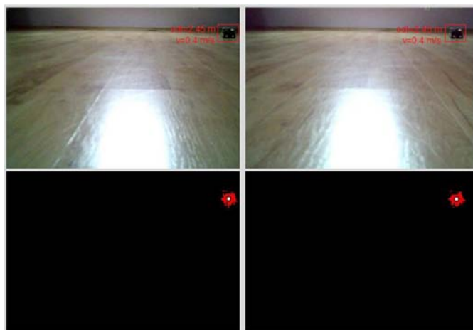
Fig. 9. Calculation of movement parameters of object, detection of moving (object is moving in perpendicular line to the optical axis of cameras with speed of 0.4 m/s)
