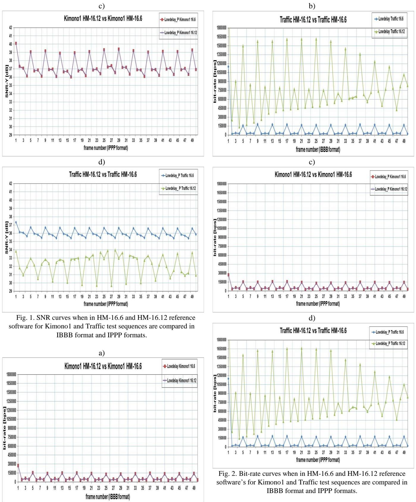
Fig. 1. SNR curves when in HM-16.6 and HM-16.12 reference software for Kimono1 and Traffic test sequences are compared in IPBB format and IPPP formats.
