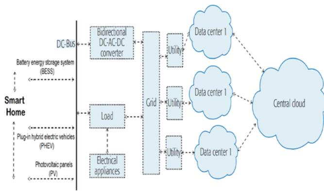
Fig. 1 Integration of nano-grid and cloud with smart buildings [1].
