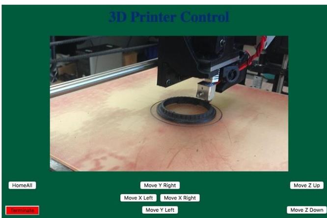
Fig. 7. GUI screenshot of live feed with print in progress.
