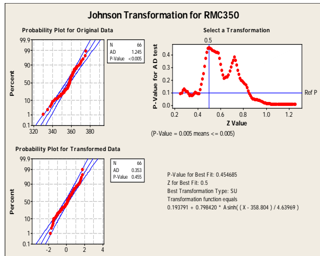
Fig. 4 Probability Plots for the Johnson Transformed data of Concrete Strength
