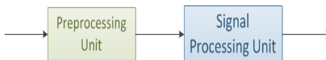
Fig. 4. The parts of EEG measurement unit. The preprocessing unit gets the raw measurement data and preprocess it. The signal processing unit is responsible for the actual evaluation of the preprocessed data.
