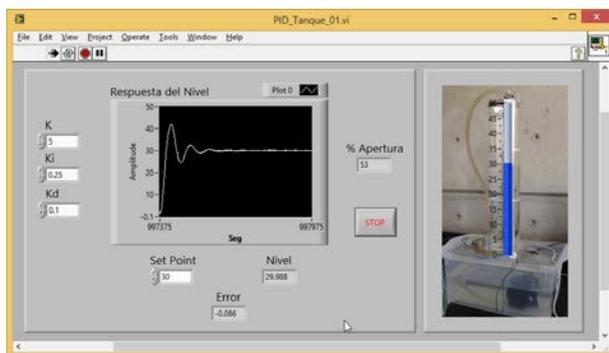
Fig. 26 Level System response with a PID controller ( $K_p = 5$ ,  $K_i = 0.25$  and  $K_d = 0.1$ .)
