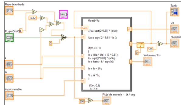
Fig. 9 Block diagram of a Level System model
