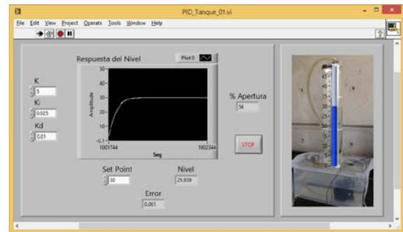
Fig. 28 Level System response with a PID controller ( $K_p = 5$ ,  $K_i = 0.025$  and  $K_d = 0.01$ .)
