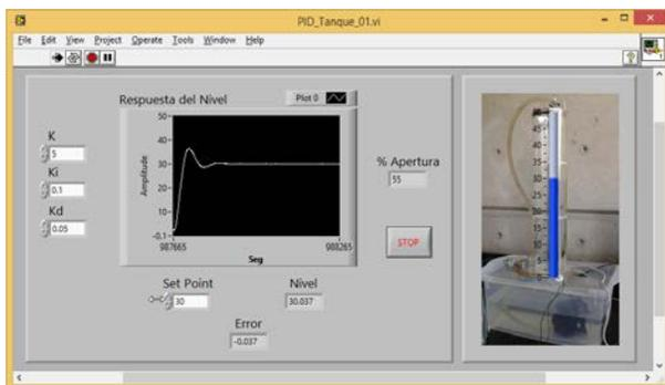
Fig. 25 Level System response with a PID controller ( $K_p = 5$ ,  $K_i = 0.1$  and  $K_d = 0.05$ .)
