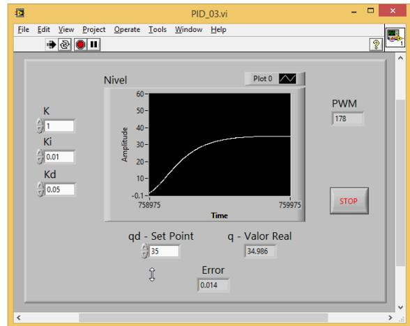
Fig. 22 Level System response with a PID controller ( $K_p = 1$ ,  $K_i = 0.1$  and  $K_d = 0.5$ .)
