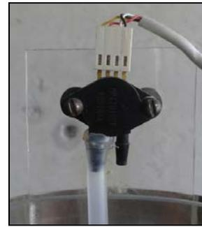
Fig. 3 MPX2010DP pressure sensor
