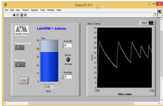
Fig. 15 VI using a RC circuit and Arduino with different control limits and hysteresis
