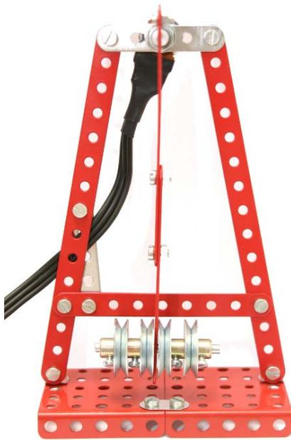
Fig. 7 Measurements of deflection of roller
