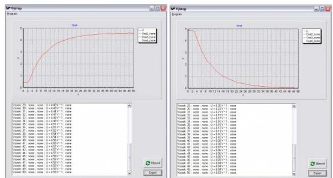
Fig. 10 Measurement of charging and discharging of capacitor
