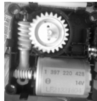
Fig. 4 DC motor Kit with worm gear reducer built-in
