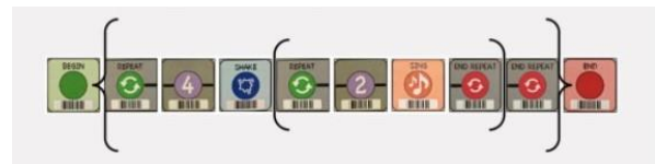
Fig. 2 Nested loops in KIBO environment. The inner loop REPEAT 2 TIMES is nested in the outer loop REPEAT 4 TIMES.
