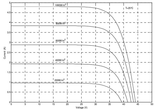
Fig. 9 Simulated I-V curves of PV module influenced by solar illumination
