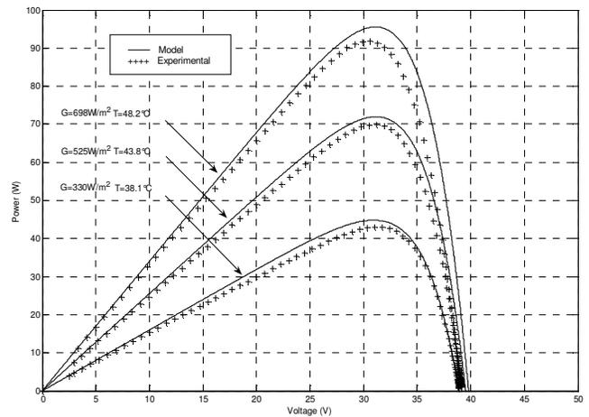
Fig. 12 Simulated P-V curves of PV module, (model results with experimental measurements), for different values of illumination and temperature.
