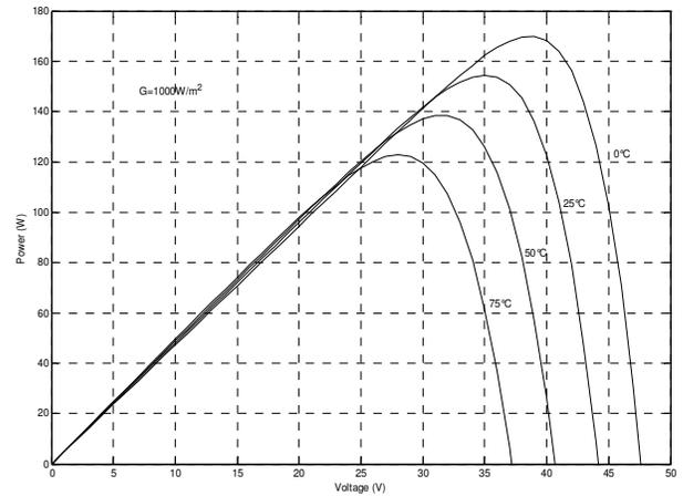
Fig. 8 Power versus voltage curves influence by temperature
