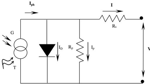
Fig. 2 the circuit diagram of the PV model.
