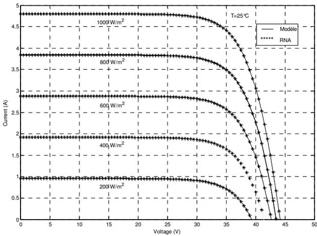
Fig. 18 Simulated I-V curves of PV module, (the model results with the results of RNA), for different values of the solar illumination at T=25°C.
