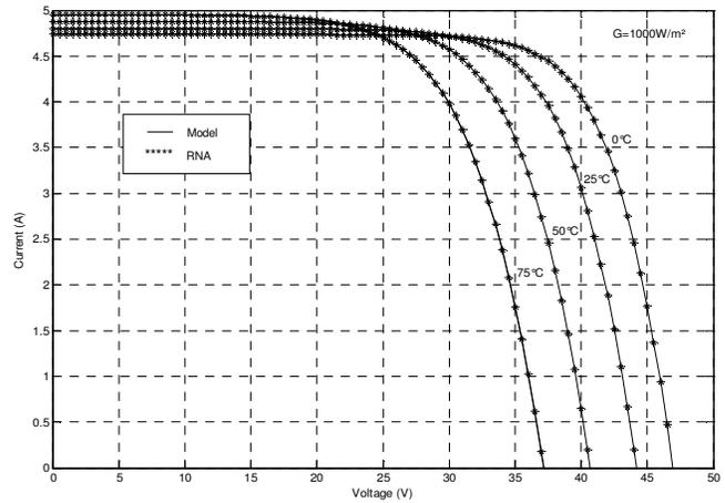
Fig. 14 Simulated I-V curves of PV module, (the model results with the results of RNA), for different values of temperature at  $G=1000W/m^2$
