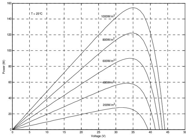
Fig. 10 Power versus voltage curves influence by the solar illumination
