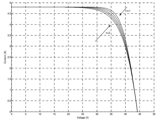
Fig. 5 Effect of diode ideality factor (1000W/m<sup>2</sup>, 25°C)
