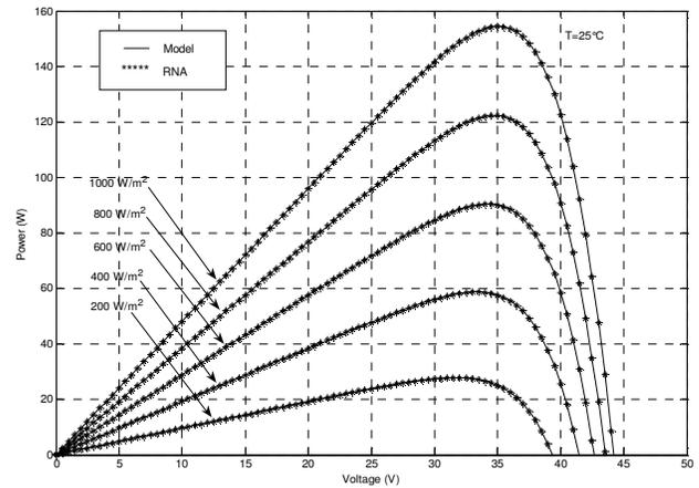
Fig. 20 Simulated P-V curves of PV module, (the model results with the results of RNA), for different values of the solar illumination at T=25°C.
