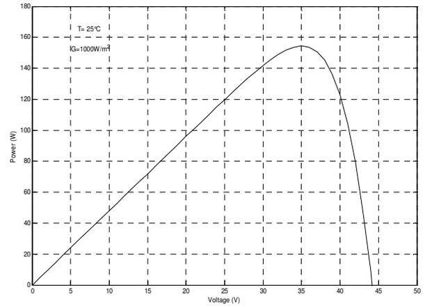
Fig. 4 P-V Curve of PV panel
