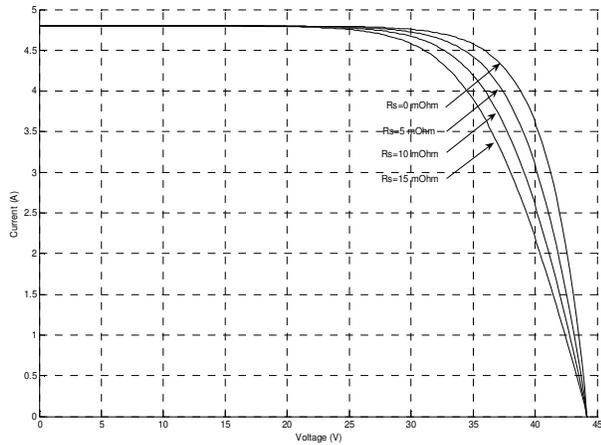
Fig. 6 Effect of series resistances ( $1000W/m^2$ ,  $25^\circ C$ )
