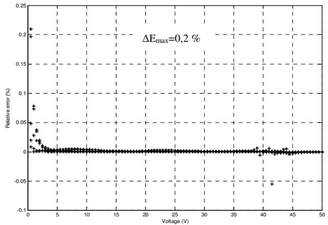
Fig. 21 The percentage of relative error in the output power of the fig. 20.
