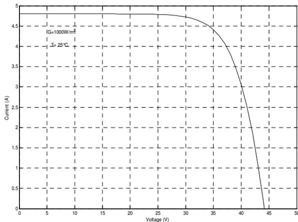
Fig. 3 I-V Curve of PV panel
