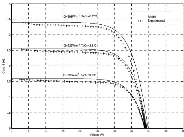
Fig. 11 Simulated I-V curves of PV module, (model results with experimental measurements), for different values of illumination and temperature.
