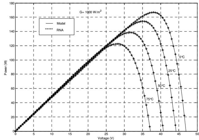
Fig. 16 Simulated P-V curves of PV module, (the model results with the results of RNA), for different values of temperature at  $G=1000W/m^2$
