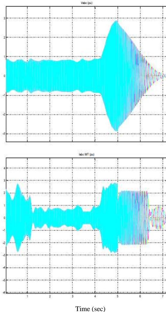
Fig. 4 The overvoltage at bus (WT) due to the ferroresonance.
