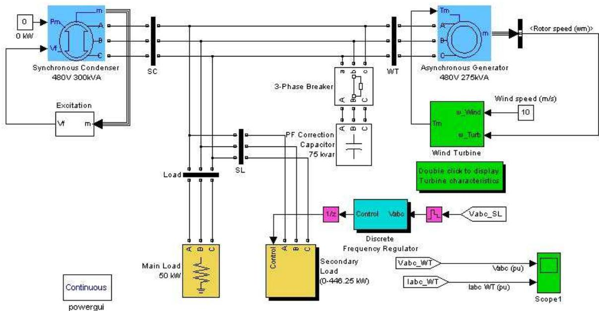
Fig.2. Simulink model for distributed resource islanded.
