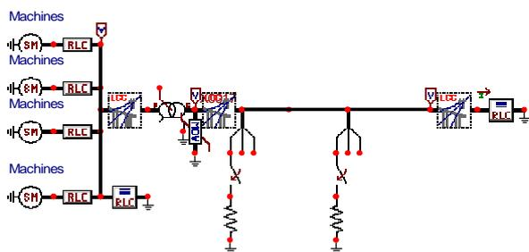
Fig. 16. Model of MV circuit, the cable feeding the transformer is replaced with a line.
