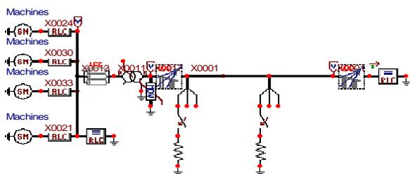
Fig 5. Model of a medium voltage network
