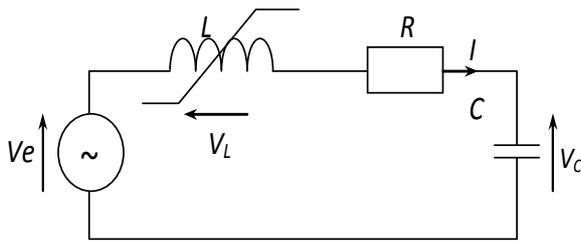
Fig. 1. Typical circuit may produce the ferroresonance.
