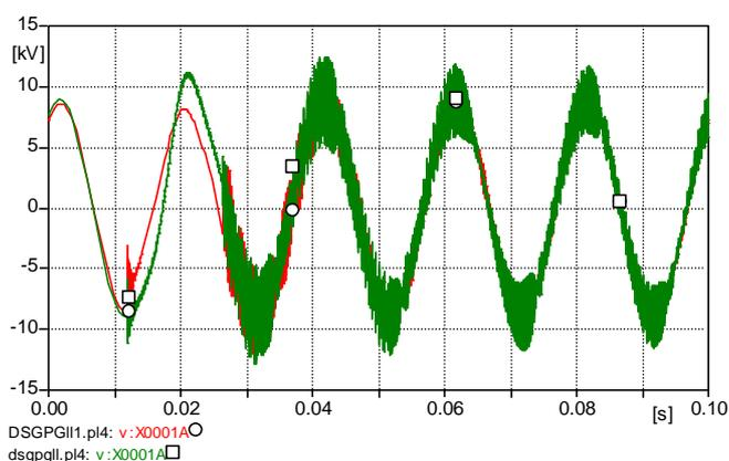
Fig. 17. Comparison between the variation of phase voltage A, in the case of cable feeding the transformer, and the case when the cable is replaced with a power line.
