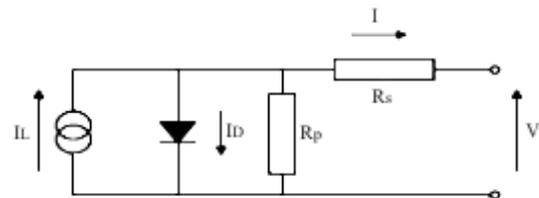
Fig. 3 - Equivalent circuit of a solar cell
