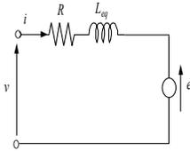
Fig. 2 – Equivalent circuit of isotropic PM brushless machine
