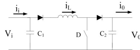
Fig. 5 – Circuit diagram of PV DC-DC converter system
