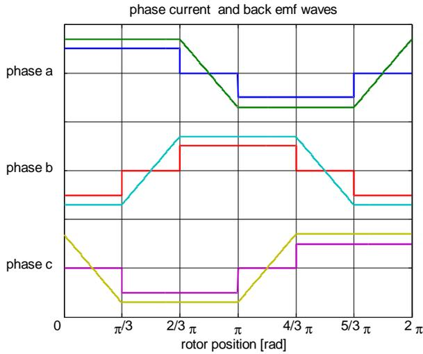
Fig. 1 – Phase currents and back EMF waves of a PM brushless dc machine
