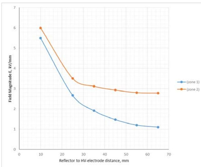
Fig. 13 Electric field E vs. the distance between the reflector and the HV-electrode
