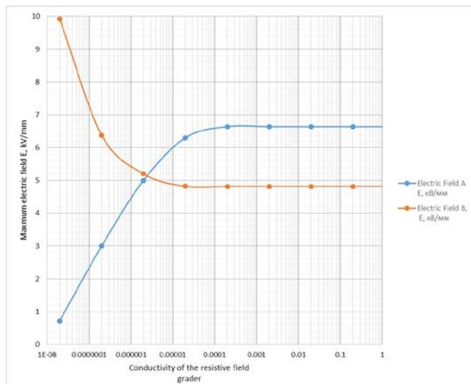
Fig. 16. Maximum electric field vs. conductivity of grading tube
