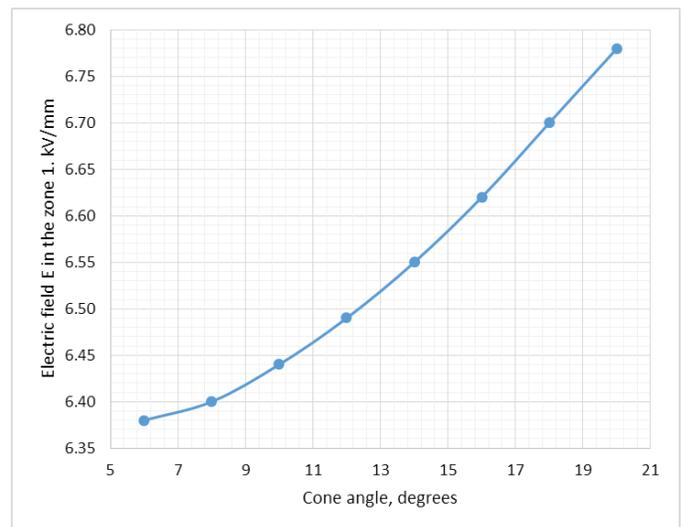
Fig. 11 The electric field E in zone 1 vs. angle of reflector cone in degrees.
