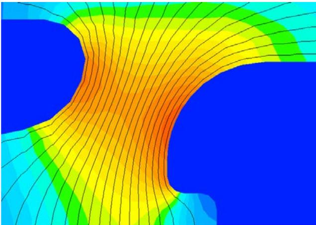
Fig. 12 Electric field between reflector and the HV-electrode. The distance is 65 mm. The most dangerous region is shown in orange color
