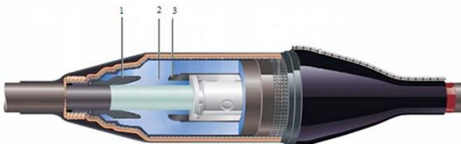
Fig. 6 Elements of the stress cone: 1 - left side reflector; 2 - main insulating body; 3 - high-voltage electrode
