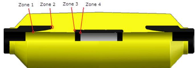
Fig. 7 The problem zones to minimize electric field: 1 – the edge of the semi-conductive layer over the insulation, 2 – reflector's edge, 3 – the edge of HV-electrode, 4 – edge of connector.
