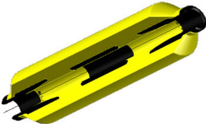
Fig. 5 The stress cone of a HV cable joint
