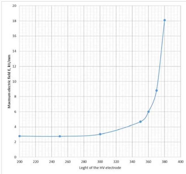
Fig. 8 The electric field E vs. length of HV-electrode
