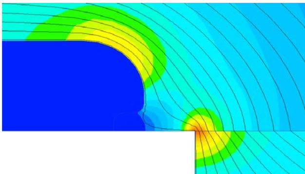
Fig. 9 The field pattern at the edge of HV-electrode (zone 3)
