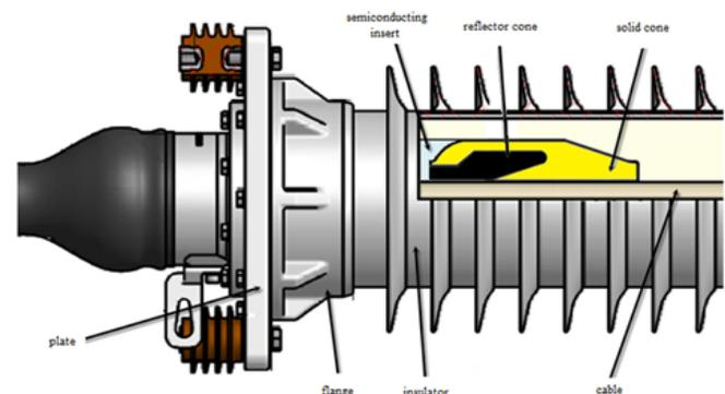
Fig. 1. Cable termination with a stress cone
