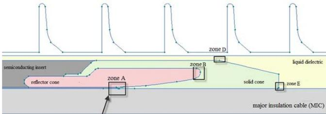
Fig. 2. Geometric design model stress cone
