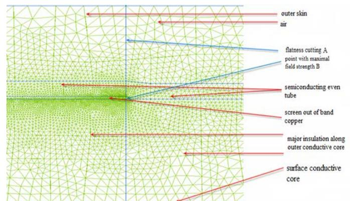
Figure 12 Calculation model cutting
