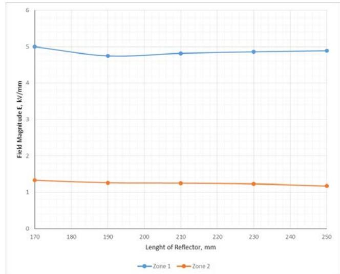
Fig. 10 Field in zones 1 and 2 vs. the length of reflector
