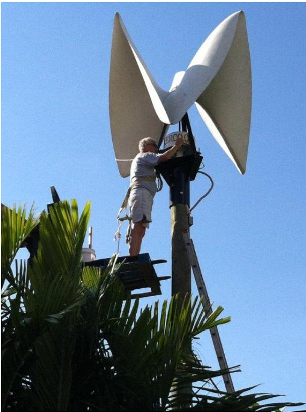
Fig. 1 Analyzed wind turbine with vertical axis helical type.
