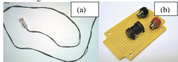
Figure 4(a) CNT based ethernet cable [27] (b) CNT wire wound on a non-magnetic core [27] [Image reproduced by permission of John Wiley & sons].
