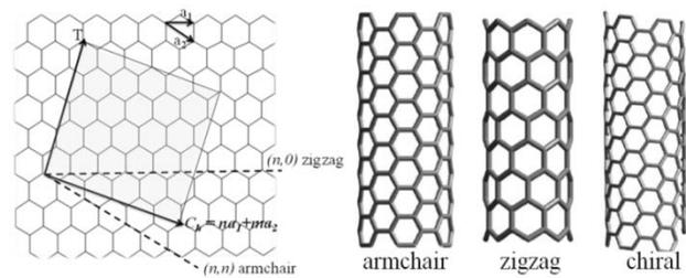
Figure 3 A sheet of graphene rolled to illustrate different types of SWCNTs [ © 2010 Choudhary V, Gupta A. Published in [15] under CC BY-NC-SA 3.0 license. Available from: <http://dx.doi.org/10.5772/18423> ].
