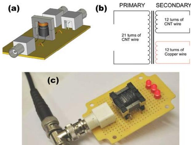
Figure 5(a) 3D schematic of the transformer [32] (b) Illustration of the windings [32] (c) Device in operation [32]. [Image reproduced by permission of John Wiley & Sons]
