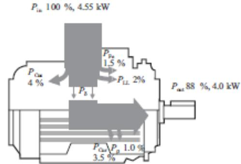
Figure 1. Sankey diagram of a 4 kW two-pole induction motor.  $P_{Fe}$ , iron losses;  $P_{Cus}$ , resistive losses of the stator;  $P_{ad}$ , additional losses;  $P_{\delta}$ , air-gap power; resistive losses of the rotor;  $P_p$ , friction losses[1][image reproduced by permission of John Wiley & sons]
