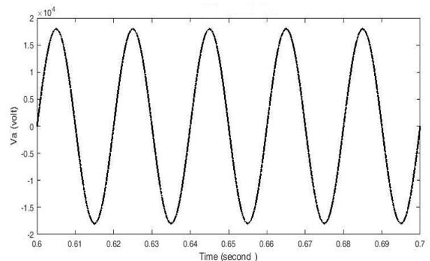
Fig.3.  $V_a$  at the grid terminal
