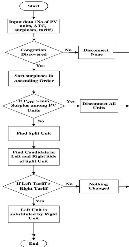
Fig. 1. Flow chart for proposed knapsack greedy algorithm
