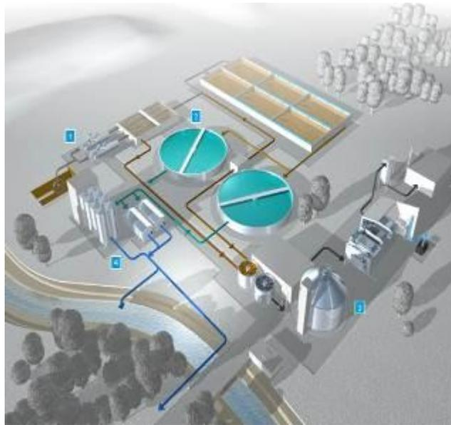
Fig. 2: Schematic presentation of water purification in MWTP (1-Mechanical preliminary treatment, 2 – Sedimentation, 3 - Sludge treatment, 4 - Microscreening, filtration) [9]
