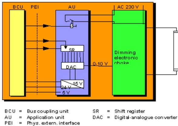
Figure 12: Detection of the Application Unit via the PEI.
