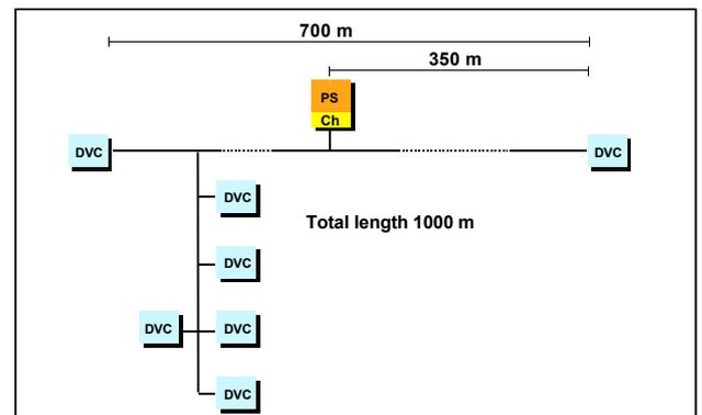
Figure 4: Permitted cable lengths.
