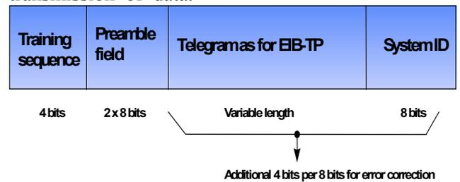
Figure 15: Additional information included in the telegram due to EIB Power Line.
