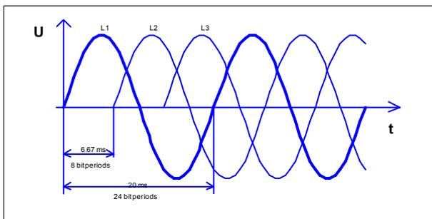
Figure 14: Phase coupling.
