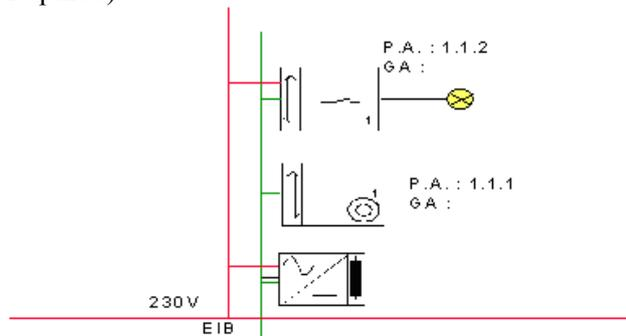
Figure 2: A minimum TP EIB installation.
