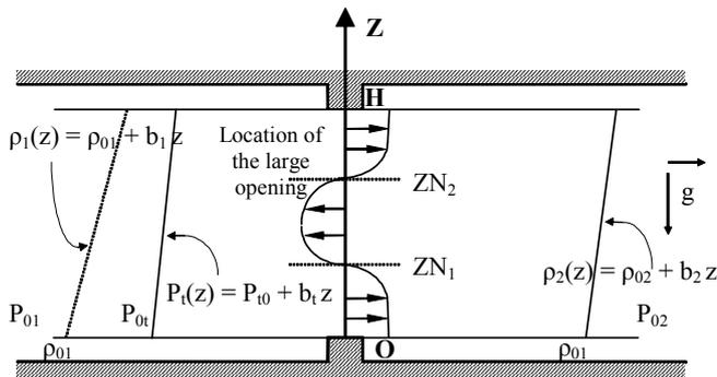
Figure 18: General problem of gravitational flow through a large vertical opening (based on Vandeale et al 1989).
