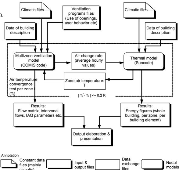
Figure 19: The introduced procedure of thermal and infiltration coupling.
