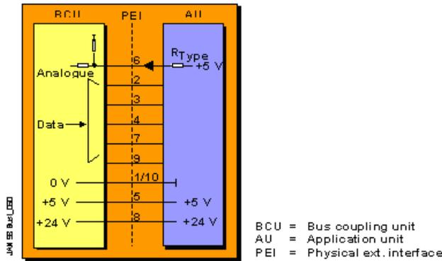
Figure 11: Interface between BCU and Application Unit.
