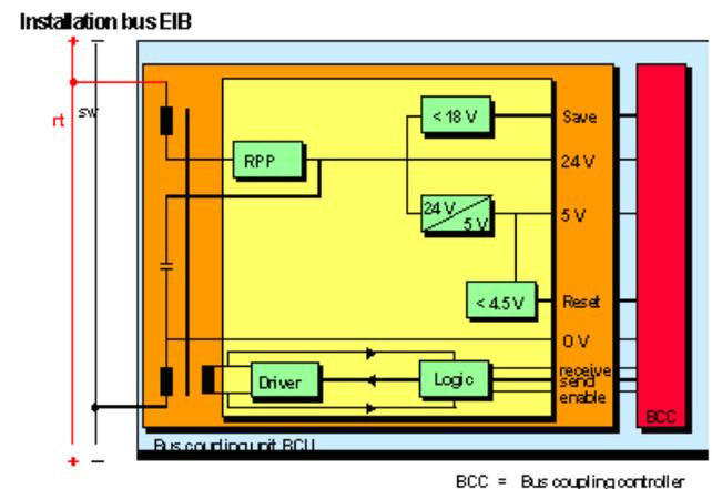
Figure 10: Bus Coupling Unit.
