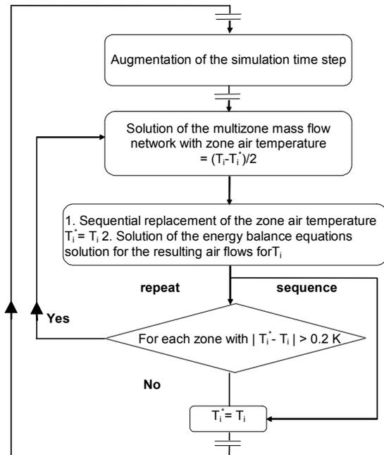
Figure 20: Flow chart of sequential coupling procedure.
