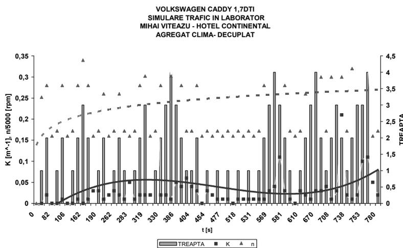
Fig. 17 Coefficient k variation versus time in experimental simulation of traffic for Volkswagen Caddy 1.7 DTI (air-conditioned unit off)
