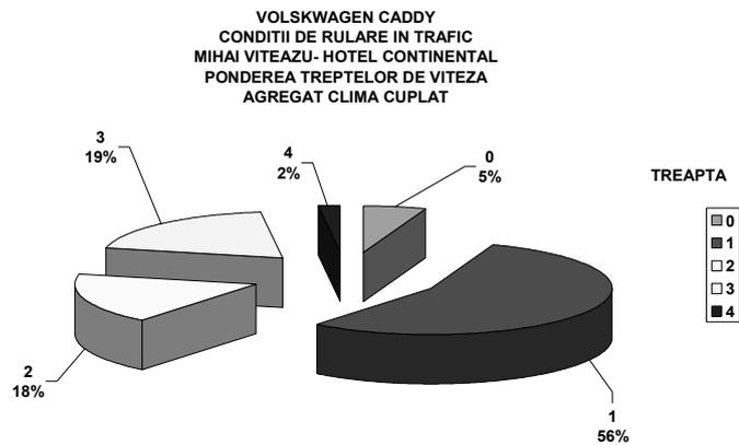
Fig. 8 Percentage of gears used for Volkswagen Caddy 1.7 DTI running in traffic (air - conditioned unit on)
