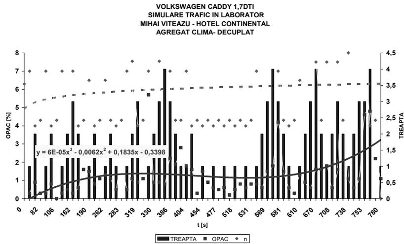
Fig. 16 Opacity variation versus time in experimental simulation of traffic for Volkswagen Caddy 1.7 DTI (air-conditioned unit off)
