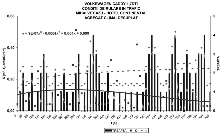
Fig. 13 Coefficient k variation versus time, for 1.7 DTI Volkswagen Caddy running in traffic (air - conditioned unit off)
