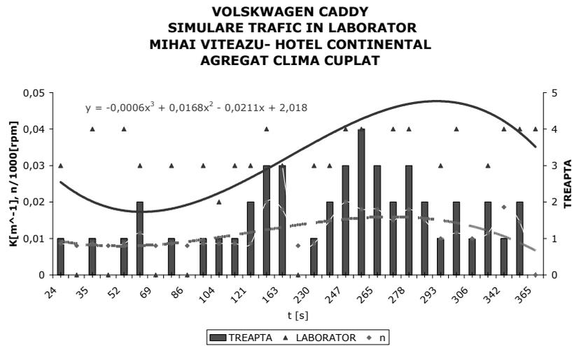
Fig. 10 Coefficient k variation versus time in experimental simulation of traffic for Volkswagen Caddy 1.7 DTI (air-conditioned unit on)
