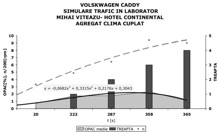
Fig. 11 Opacity average variation versus time in experimental simulation of traffic for Volkswagen Caddy 1.7 DTI (air-conditioned unit on)
