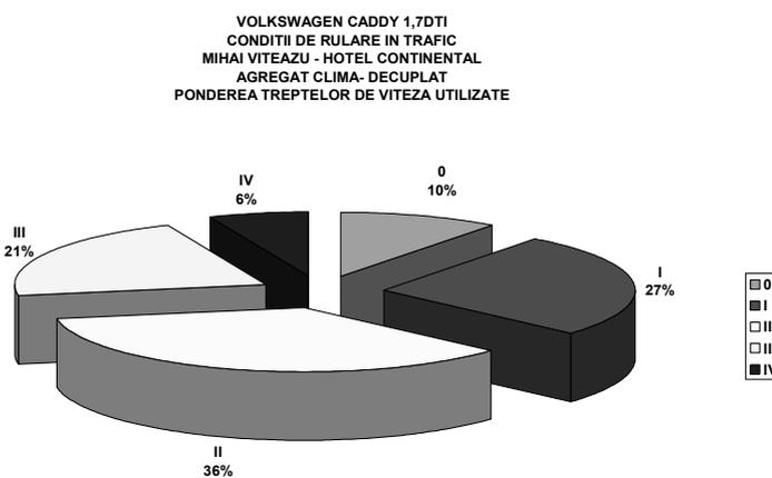
Fig. 15 Percentage of gears used for Volkswagen Caddy 1.7 DTI running in traffic (air - conditioned unit off)
