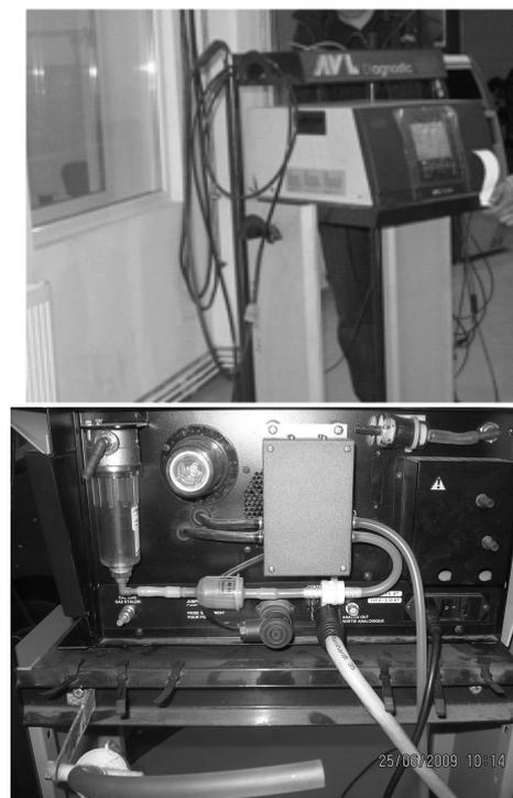
Fig. 2 AVL Dicom 4000 gas analyzer
