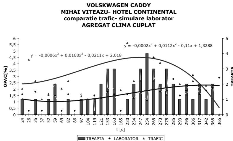
Fig. 19 Opacity variation versus time, for Volkswagen Caddy 1.7 DTI running in traffic and experimental simulation of traffic (air conditioned unit on)
