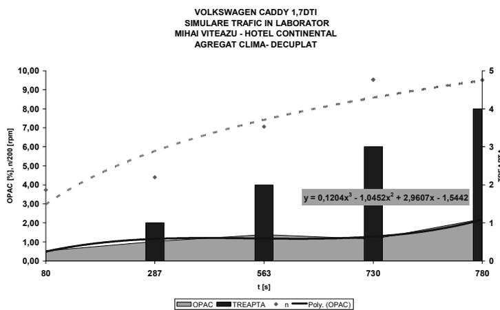
Fig. 18 Opacity average variation versus time in experimental simulation of traffic for Volkswagen Caddy 1.7 DTI (air-conditioned unit off)
