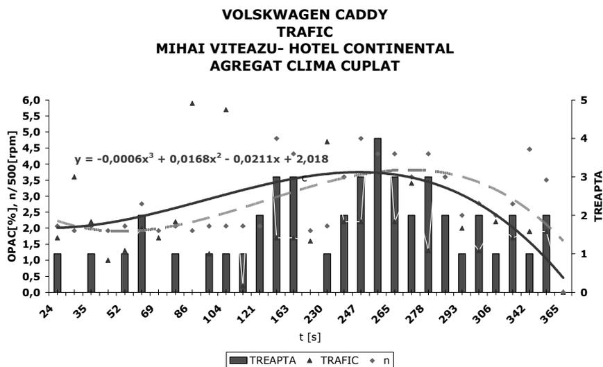
Fig. 5 Opacity variation versus time, for 1.7 DTI Volkswagen Caddy running in traffic (air - conditioned unit on)
