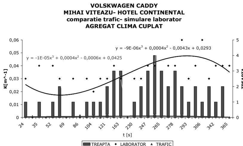
Fig. 20 Coefficient k variation versus time, for Volkswagen Caddy 1.7 DTI running in traffic and experimental simulation of traffic (air conditioned unit on)
