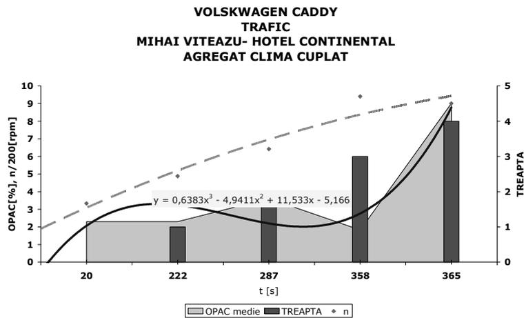
Fig. 7 Average opacity variation versus time, for 1.7 DTI Volkswagen Caddy running in traffic (air-conditioned unit on)
