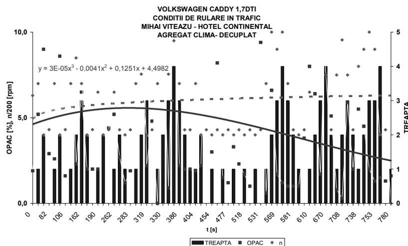
Fig. 12 Opacity variation versus time, for 1.7 DTI Volkswagen Caddy running in traffic (air - conditioned unit off)
