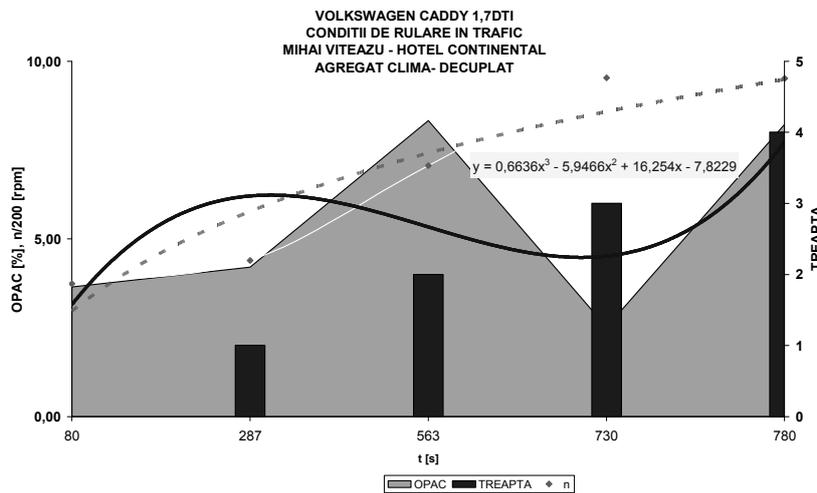
Fig. 14 Average opacity variation versus time, for 1.7 DTI Volkswagen Caddy running in traffic (air - conditioned unit off)
