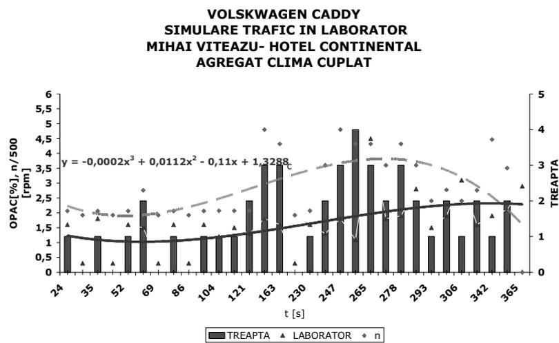
Fig. 9 Opacity variation versus time in experimental simulation of traffic for Volkswagen Caddy 1.7 DTI (air-conditioned unit on)
