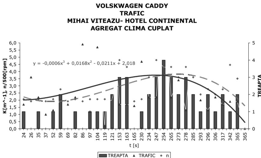
Fig. 6 Coefficient k versus time, for 1.7 DTI Volkswagen Caddy running in traffic (air - conditioned unit on)
