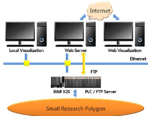
Fig. 17 block scheme of SRP measurement system – real technology of research polygon, PLC of B&R X20 CP1484, some PCs with local visualization, Web server, and Web visualization
