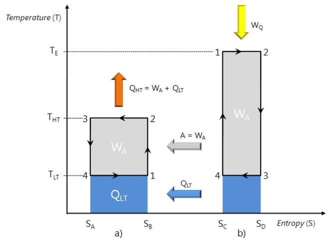
Fig. 6 temperature/entropy diagram includes the reversible Carnot cycle (a) and the clockwise Carnot cycle (b) – absorption heat pumps
