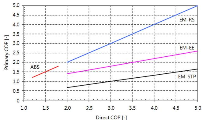
Fig. 11 primary COP graphical dependence on direct COP for various kinds of heat pumps (ABS, EM-RS, EM-EE, and EM-STP)
