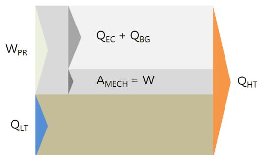
Fig. 9 balance diagram of compressor-based heat pump powered by explosion engine
