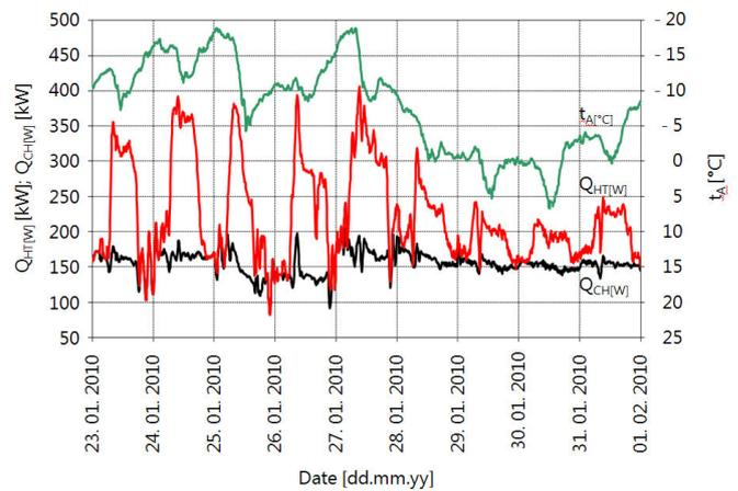
Fig. 16 graphical characteristics of total heat power  $Q_{HT[W]}$  (air-conditioning and central heating; red line), heat power for central heating  $Q_{CH[W]}$  (central heating; black line), and ambient air temperature  $t_{A[^{\circ}\text{C}]}$  (grey line) the BRP heat pumps at extreme conditions (January 2010/February 2010)
