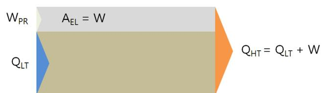
Fig. 8 balance diagram of compressor-based heat pump powered by electric energy, produced via non-thermal power-plants (i. e. water-power, wind-power, and photovoltaic-power ones)
