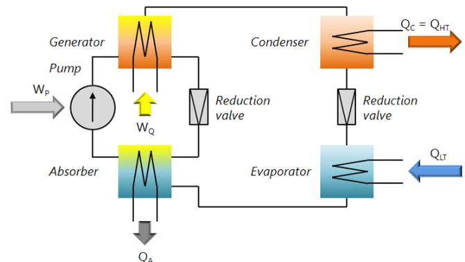
Fig. 4 block diagram of absorption heat pump with its important parts inside the first circuit (pump, generator, reduction valve, and absorber), inside the second circuit (condenser, reduction valve, and evaporator), and labels of quantities
