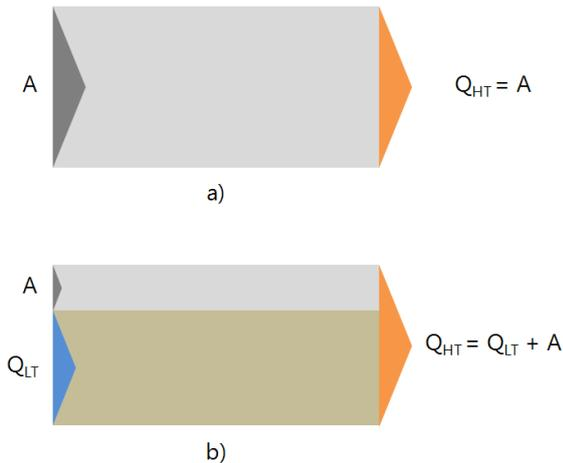
Fig. 1 comparison between direct heating (a) and heating via heat pump (b) – the case of ideal lossless energy balance
