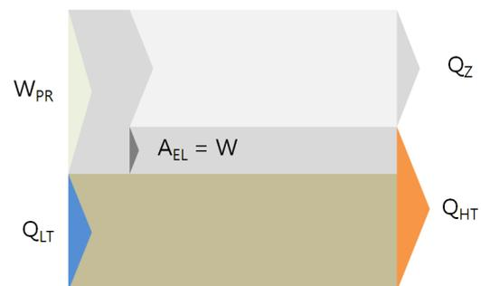
Fig. 7 balance diagram of compressor-based heat pump powered by electric energy, produced via thermal power-plant (condenser type)
