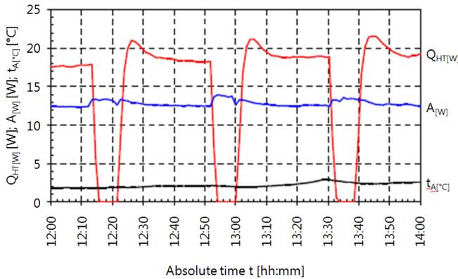
Fig. 2 graphic illustration of practical effectiveness of badly structurally designed heat pump – an activity time period of this heat pump is two hours
