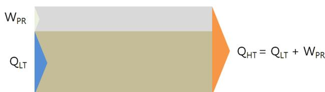
Fig. 10 balance diagram of absorption heat pump
