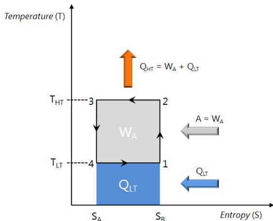
Fig. 5 temperature/entropy diagram of the reversible Carnot cycle for heat pumps powered by mechanical work – compressor-based heat pumps
