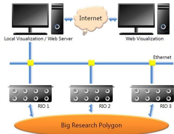
Fig. 15a block scheme of BRP measurement system – real technology of research polygon, remote I/O units, some PCs with local visualization, Web server, and Web visualization
