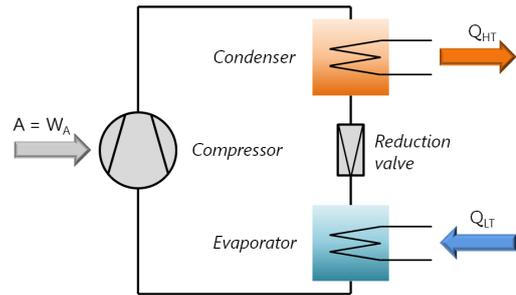
Fig. 3 block diagram of compressor-based heat pump with its important parts (compressor, condenser, reduction valve, and evaporator), and labels of quantities
