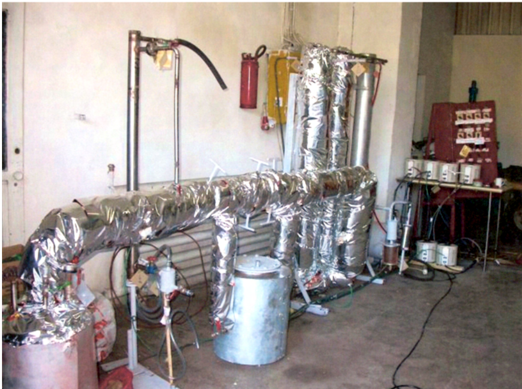
Fig. 1 Photo of the experimental plant to produce hydrogen and iron powder.
