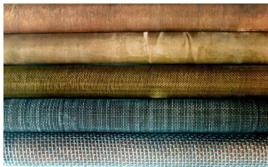
Fig. 3 Sleeves made by metallic tissues mounted on tubes
