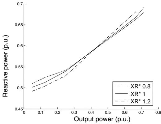
Fig.11 Variation of Reactive power with output power for different values of rotor leakage reactance.
