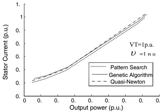
Fig.16 Variation of stator current with output power using different optimization tools.
