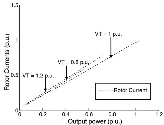
Fig.14 Variation of rotor current with output power for different values of terminal voltage.
