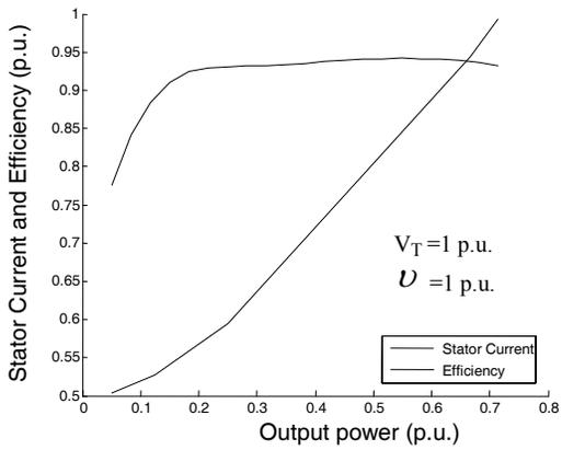
Fig.5 Variation of stator current and efficiency with output power.
