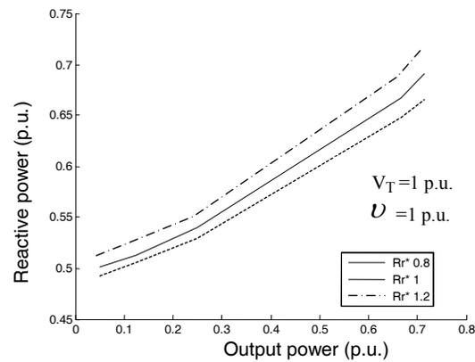
Fig.9 Variation of Reactive power with output power for different values of rotor resistance.
