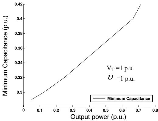
Fig.7 Variation of minimum capacitance with output power.
