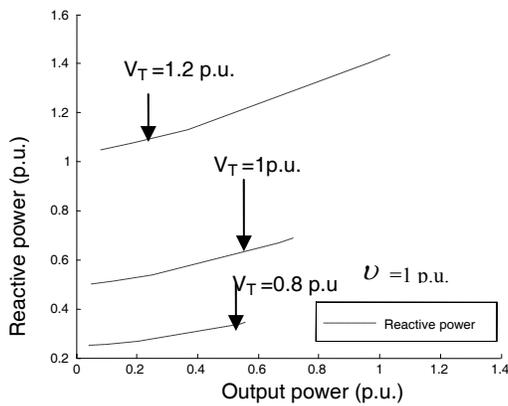
Fig.12 Variation of reactive power with output power for different values of terminal voltage.
