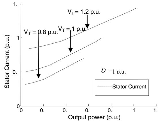
Fig.13 Variation of stator current with output power for different values of terminal voltage.
