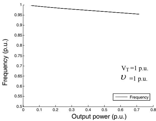
Fig.6 Variation of frequency with output power.
