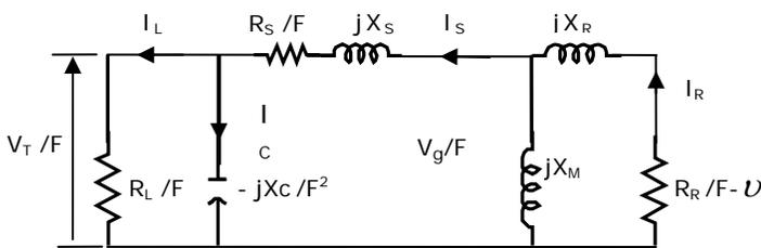
Fig.1 Per-phase equivalent circuit of SEIG
