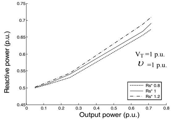
Fig.8 Variation of Reactive power with output power for different values of stator resistance.
