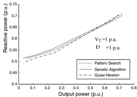
Fig.15 Variation of reactive power with output power using different optimization tools.
