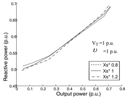
Fig.10 Variation of Reactive power with output power for different values of stator leakage reactance.
