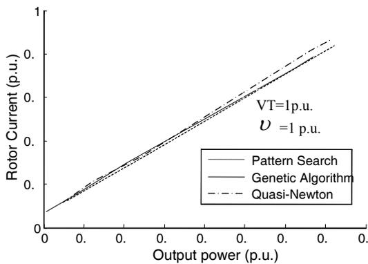
Fig.17 Variation of rotor current with output power using different optimization tools.
