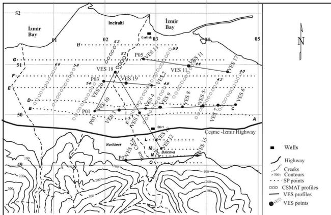
Fig. 2 Locations of SP, resistivity and CSAMT surveying profiles.
