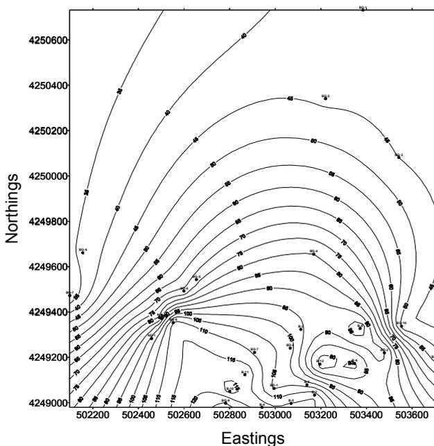
Fig. 3 Temperature distribution at 40 m bsl [7].
