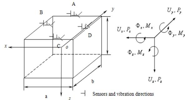
Fig. 1 Degree-of-freedom of a massive foundation vibration
