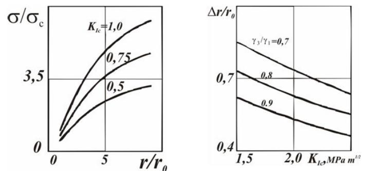
Fig. 4. Dependence of the last failure zone position from the stresses acting within the rock mass (left) and the radial length one of the first zone of failure from the rock fracture toughness (right)
