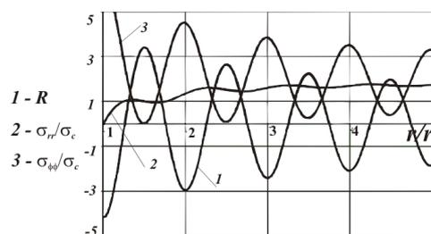
Fig. 2. Oscillating character of the stresses and R - functions in the rock mass surrounding the underground opening
