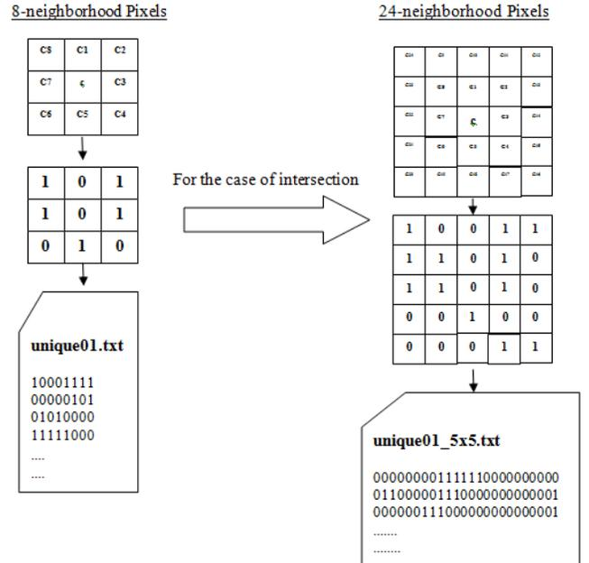
Fig. 15. Converting cells' values into text files
