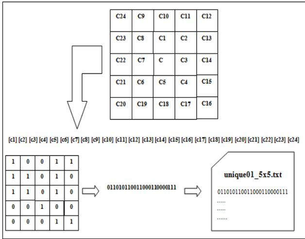
Fig. 13. Process of determining 24 surrounding cells
