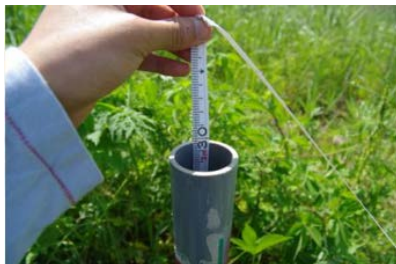
Fig. 7 Measurement of flow depth
