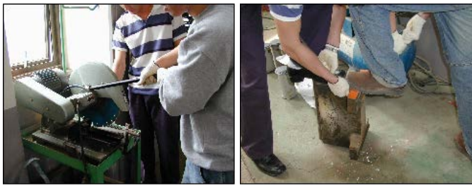
Fig. 5 Process of marking the scales to the reinforced bar staff
