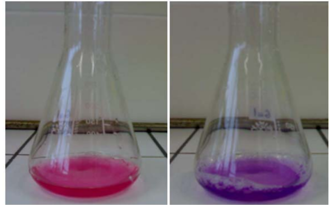
Fig.3. Colour change of tested samples by chelatometric titration – sample before titration (on the left) and sample after titration (on the right)
