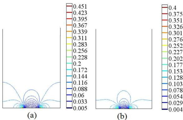
Fig. 6. Contour plot of pressure ( $MPa$ ) at  $t = 1\text{ s}$  in the granular material at the bottom part of the flat-bottomed silo with two different outlet widths: (a)  $0.012\text{ m}$ ; (b)  $0.08\text{ m}$ .
