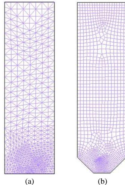
Fig. 4. Domain mesh of the two silos: (a) flat-bottomed silo; (b) cone-bottomed silo.
