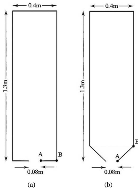
Fig. 3. Geometries of the two silos having different bottom design: (a) flat shape; (b) hopper shape.
