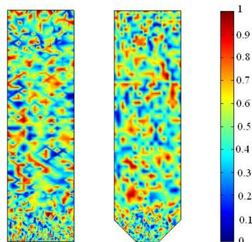
Fig. 5. Volume fraction of soybeans at initial time  $t = 0s$  in the flat-bottomed silo and the cone-bottomed silo, respectively.
