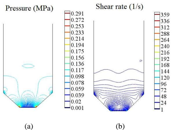
Fig. 8. Contour plot of pressure and shear rate of the granular material at the bottom part of the cone-bottomed silo at  $t = 1\text{ s}$ .
