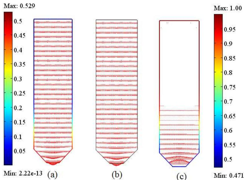
Fig. 13. Velocity vector of solid phase, mixture and air phase in the cone-bottomed silo at  $t = 1$ s.
