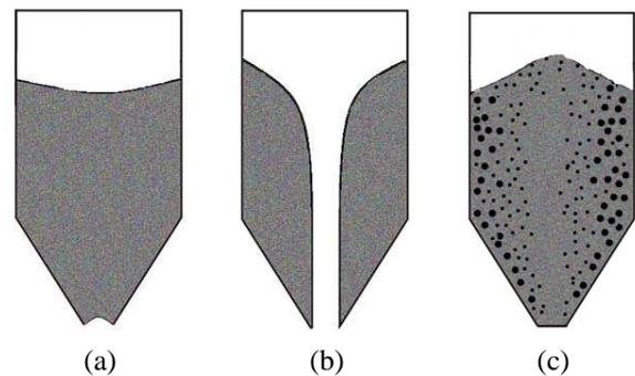
Fig. 1. Flow problems: (a) Arching; (b) Piping; (c) Segregation
