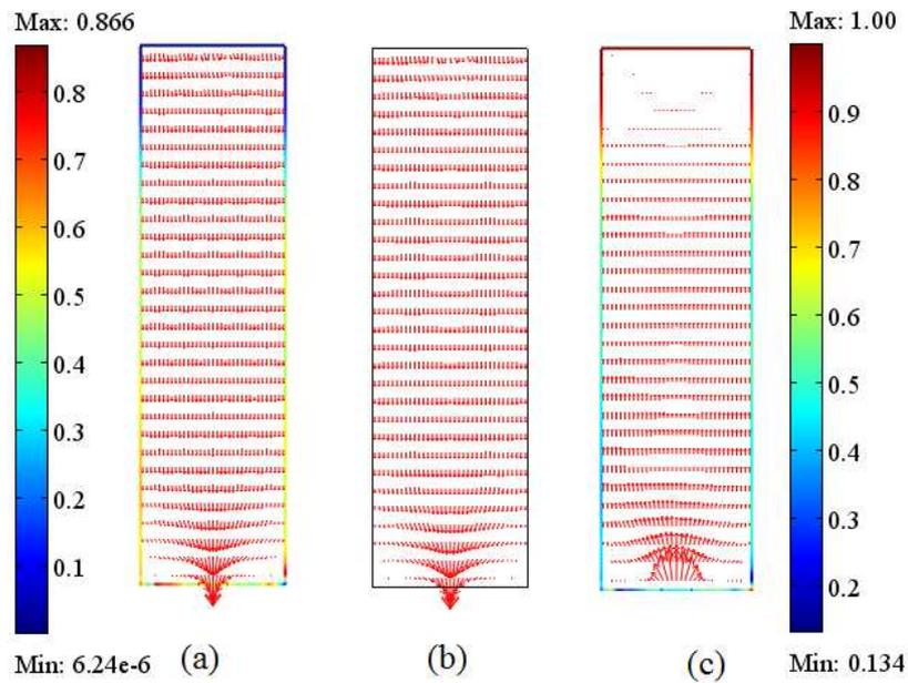
Fig. 12. Velocity vector of solid phase, mixture and air phase in the flat-bottomed silo at  $t = 1$ s.
