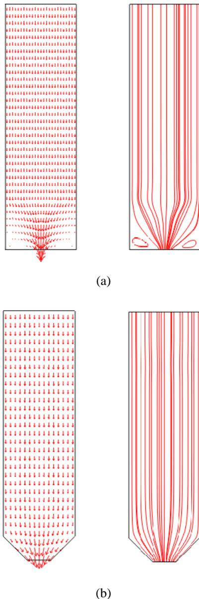
Fig. 9. Velocity vector and stream line of the granular material in both silos with the outlet width of  $0.08\text{ m}$ : (a) the flat-bottomed silo; (b) the cone-bottomed silo.
