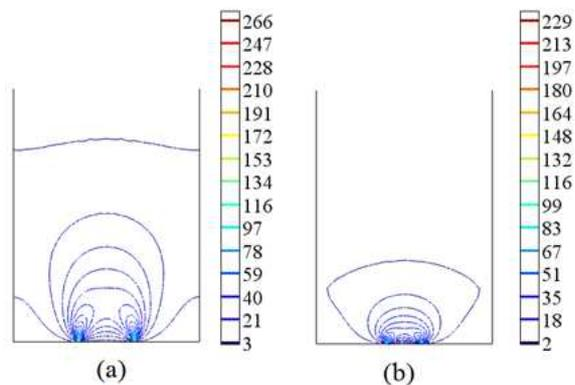
Fig. 7. Contour plot of shear rate ( $MPa$ ) at  $t = 1\text{ s}$  in the granular material at the bottom part of the flat-bottomed silo with two different outlet widths: (a)  $0.012\text{ m}$ ; (b)  $0.08\text{ m}$ .
