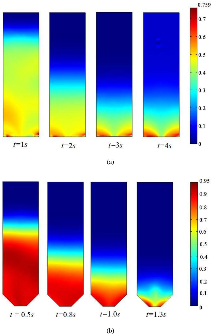
Fig. 11. Volume fraction of soybeans at different times during discharging process obtained from both silos: (a) the flat-bottomed silo; (b) the cone-bottomed silo.
