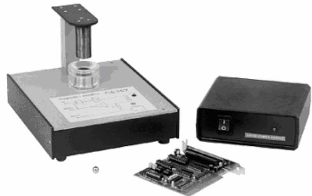
Fig. 2 The CE 152 magnetic levitation apparatus
