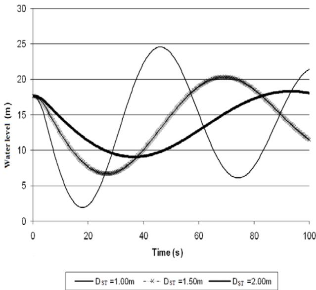
Fig. 7 Water level in the surge tank
