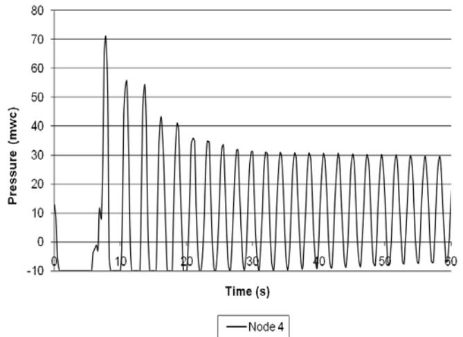
Fig. 4 Pressure in the discharge duct
