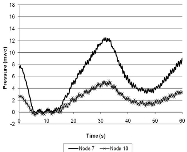
Fig.15 Pressure variation in the case of one air chamber with asymmetrical hydraulic resistance
