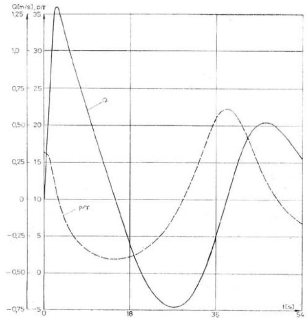
Fig. 11 Air layer pressure ( $p/\gamma$ ) and the water flow rate between air chamber and the discharge duct ( $Q$ ) [11]
