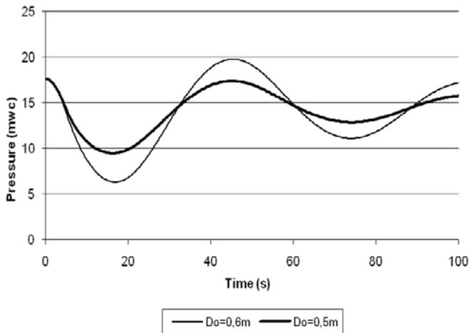
Fig. 9 Water level (pressure) in the surge tank with throttled connection duct
