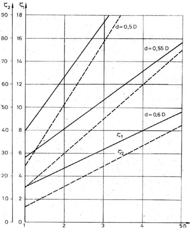
Fig. 13 Coefficients of local hydraulic resistance  $\zeta_1$  and  $\zeta_2$  as functions of the number of conical nozzles in an asymmetrical resistance device [12], [13]
