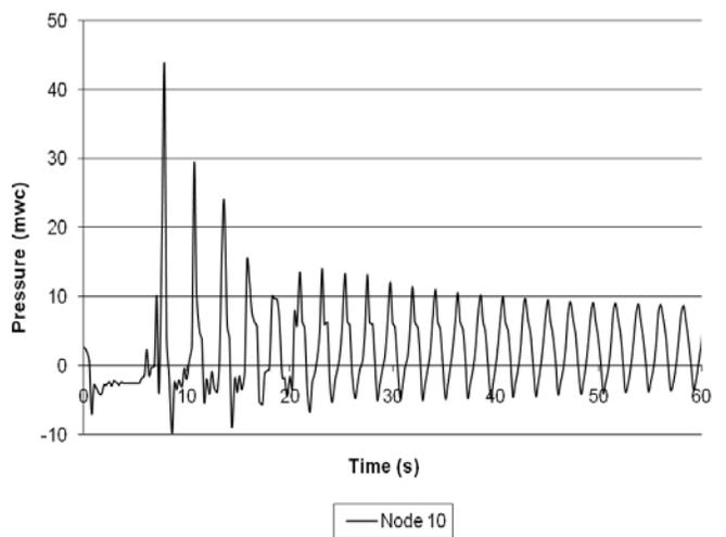
Fig. 6 Pressure in the discharge duct
