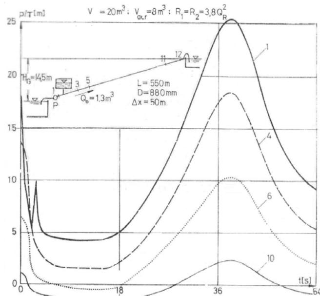
Fig. 10 Old pumping station SRP 4 Seimeni. Pressure values in the discharge duct [11]
