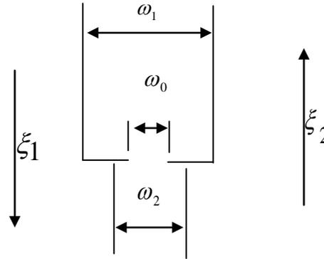
Fig. 8 The hydraulic resistance placed on the connection duct between the surge tank and the discharge duct
