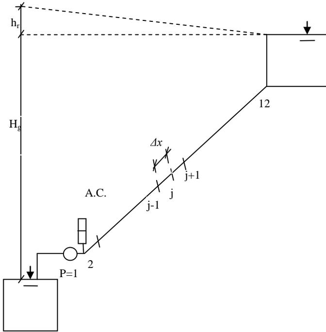
Fig.1 Pumping station with air chamber on the discharge duct
