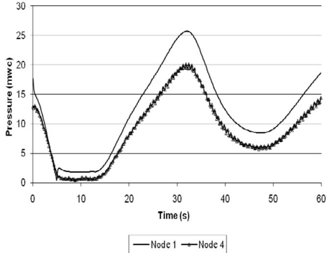
Fig.14 Pressure variation in the case of one air chamber with asymmetrical hydraulic resistance
