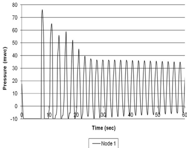
Fig. 3 Pressure in the discharge duct
